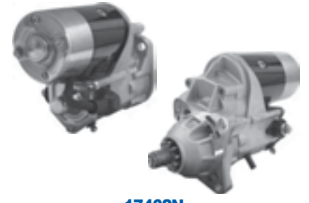
17462N Starter - Denso OSGR 2.7KW/12 Volts, CW, 11-Tooth Pinion Used on: Bobcat Skid Loader, OPE & Industrial, Clark Skid Loader Replaces: Bobcat 6667587; Denso 228000-581
