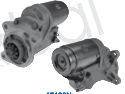
17100N Starter - Denso OSGR 1.4KW/12 Volt, CW, 10-Tooth Pinion For: Caterpillar Lift Trucks w/ Cat 1404 Engine or Continental F-163, F-227 Engines Replaces: Caterpillar 3T5649, Denso 028000-8230
