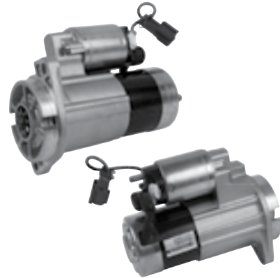
18973N Starter - Mitsubishi PMGR 12 Volt, CW, 9-Tooth Pinion
