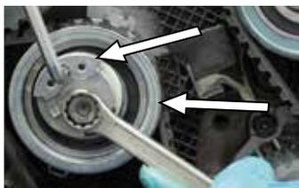
**25.** To check belt tension use the appropriate instruments that are able to provide reliable data on the tension value applied.
