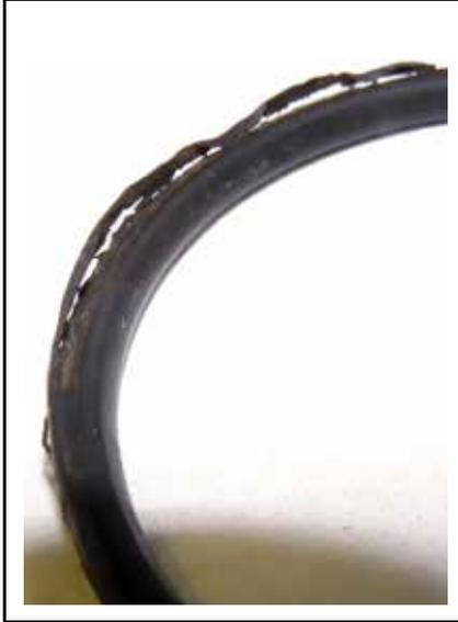
10.13 Damage caused by incorrect installation
