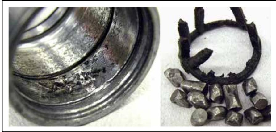
10.9 Bearing components damaged due to overload
