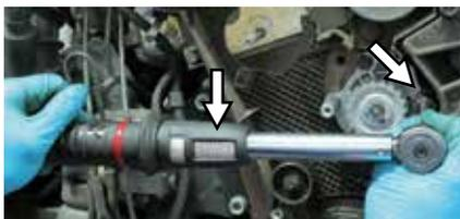
13. Strictly observe the tightening torque of the screws indicated by the manufacturer.
