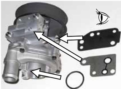
12. The mounting screws should be tightened crosswise and, before tightening them completely, **you must ensure that the pump is centered correctly and can rotate freely in its housing.**
