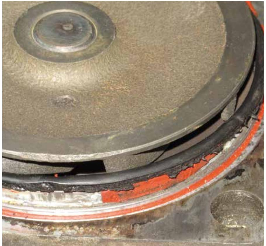
10.12 Sealant paste Sealant paste incorrectly applied on O-rings
