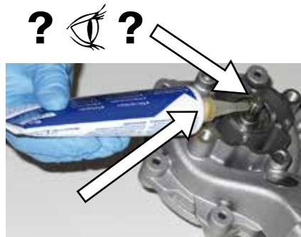
**20.** Check the condition and the proper operation of the thermostat.
