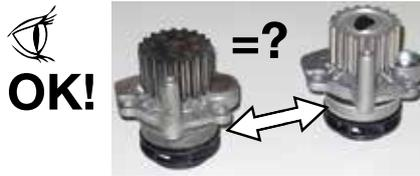
9. If the pump has a gasket, metal or other type, the sealing paste should **not be used**; the gasket supplied with the pump is adequate to ensure a perfect seal, make sure the mounting
