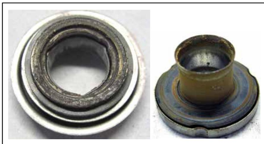
10.2 Mechanical seals damaged by unsuitable coolants
