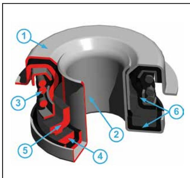
8.4 Section of a typical mechanical seal
