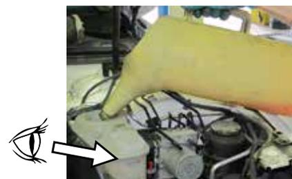
**27.** Start the engine and leave it to idle, turn on the heating in the compartment and continue to refill the coolant from the highest point of the circuit (generally the expansion tank) until the level does not drop any more, wait for the opening of the thermostat so as to properly fill also the radiator.
