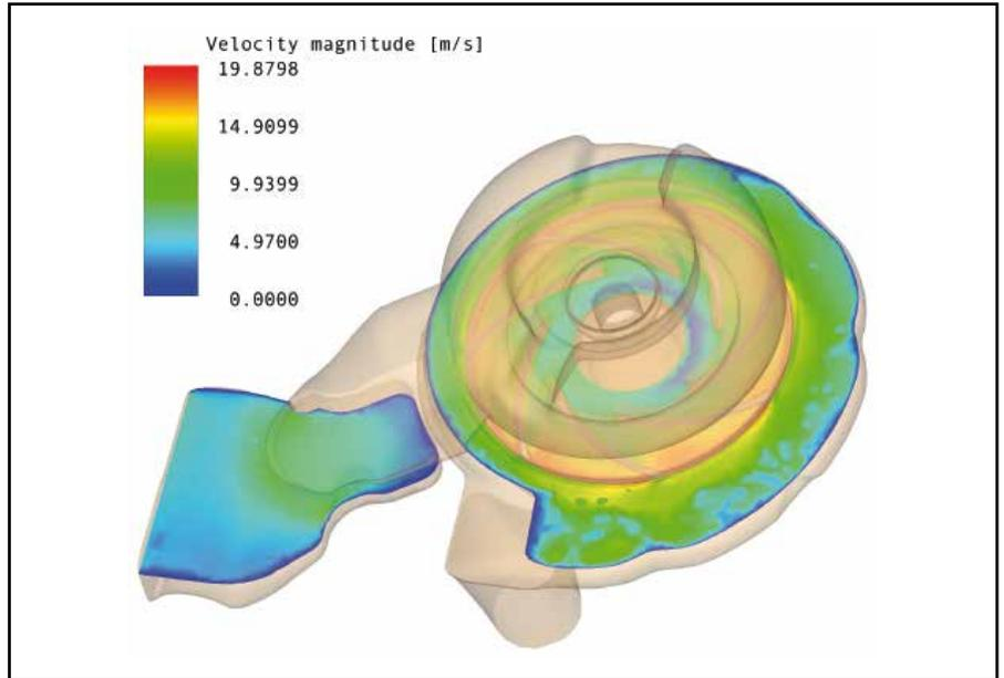
6.1 Fluid dynamics analysis of a water pump
