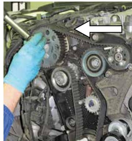
**24.** Tighten the belt respecting the value recommended by the manufacturer; avoid excessive tension, allow the engine to run
