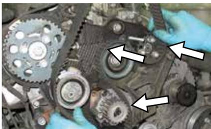
**19.** Some water pumps have gears and spline shafts as drives; ensure the good condition of the gear
