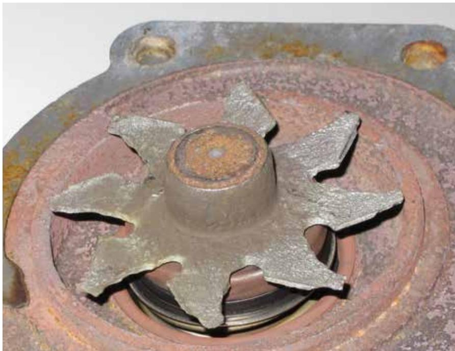
7.1 Impeller completely corroded due to incorrect fluid
