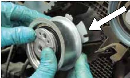
**18.** Place the belt correctly following the manufacturer's instructions, especially when this concerns the timing belt, if special tools are required, use them.
