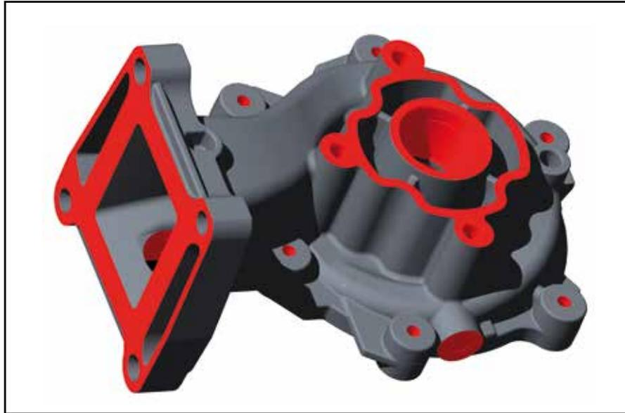
8.8 3D model of a water pump housing
