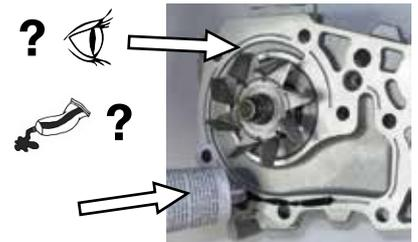
11. Each seal that has been removed should be replaced with a new one, never reuse gaskets used even if they seem in good condition.
