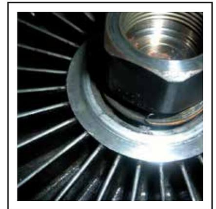
10.5 Damaged viscous coupling unit
