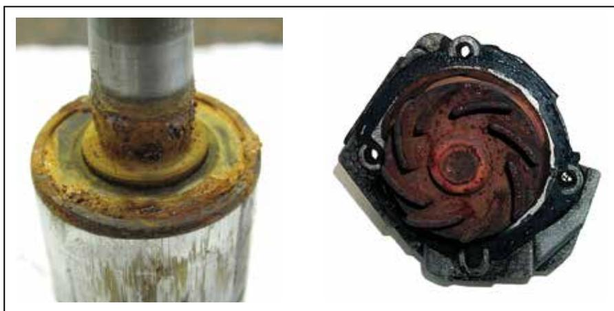
10.1 Rusted components due to unsuitable coolants
