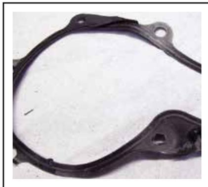
10.11 Sealant paste incorrectly applied on metal gasket
