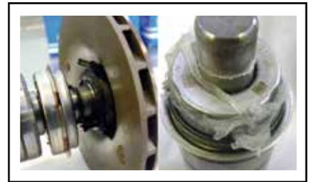
10.10 Improper use of sealing material
