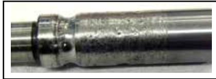
10.8 Bearing shaft damaged by excessive load
