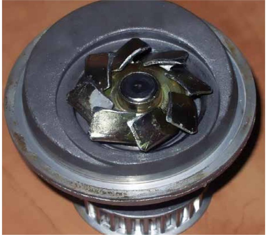
10.15 Impeller damaged by foreign object in the circuit
