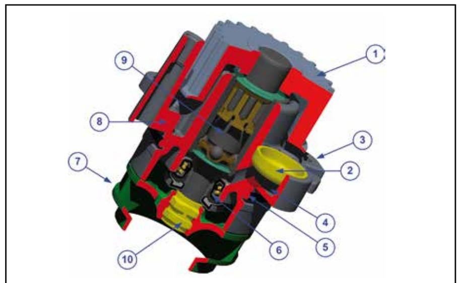
4.1 Section of a water pump and its components
