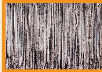
Scratch Marks on Piston Ring Running Face Caused By Foreign Particles
