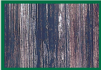
Scuffed Running Face of Piston Ring
