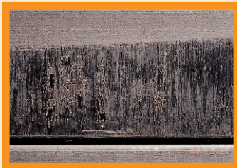
Foreign Particles Stuck on Piston Ring Running Surface
