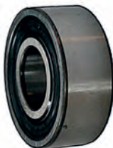
140900 5★ 62203-2RS1/C3 Ball Bearing Manufacturer: SKF ID 17.00, OD 40.00, Height 16.00
