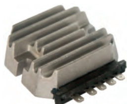
234408 Regulator/Rectifier Replacing: AM101406 14 Volt, Dist. mount. holes 61.40
