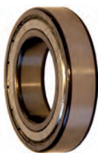
140887 FAG 6007-2ZR Ball Bearing ID 35.00, OD 62.00, Height 14.00
