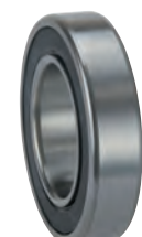
142289 6007-2RS/C3 Ball Bearing ID 35.00, OD 62.00, Height 14.00 Alternative no.: 140631
