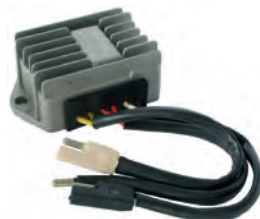
234854 Regulator/Rectifier Replacing: 434362600 14 Volt, 25 Amp, Dist. mount. holes 92.00w/ recharge response.
