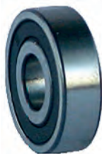
141058 609-2RS/C3 Ball Bearing ID 9.00, OD 24.00, Height 7.00
