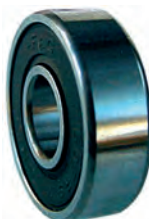
141059 FAG 627-2RS/C3 Ball Bearing ID 7.00, OD 23.00, Height 7.00
