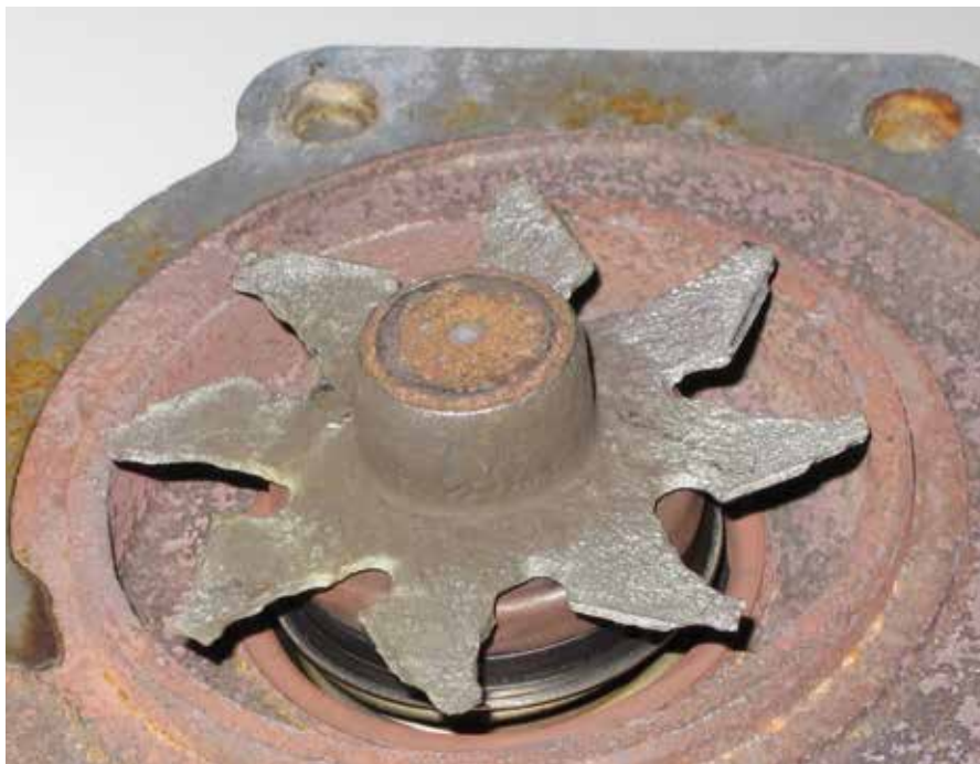
7.1 Impeller completely corroded due to incorrect fluid
