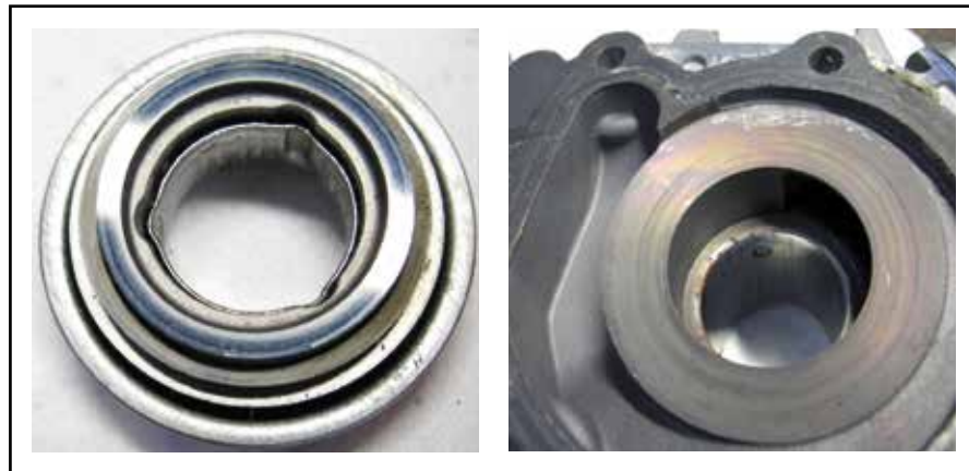
10.4 Surfaces with signs of overheating
