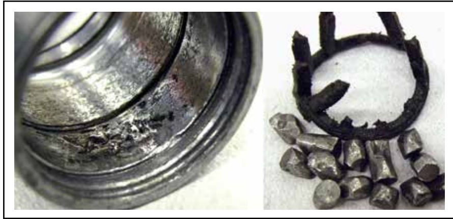
10.9 Bearing components damaged due to overload
