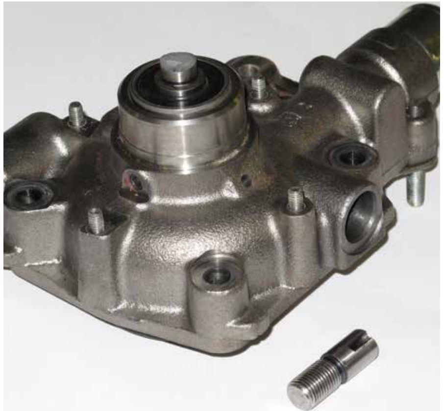
10.14 bearing shaft broken due to incorrect assembly operations
