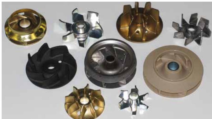
8.3 Impellers manufactured in different ways
