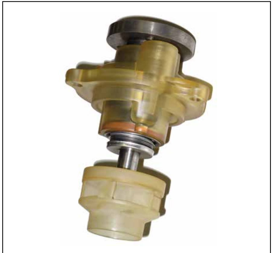
6.2 Water pump prototype with components made of resin
