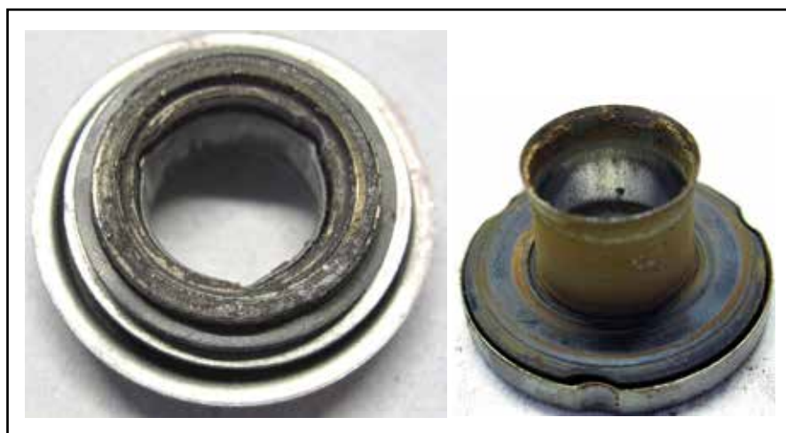
10.2 Mechanical seals damaged by unsuitable coolants
