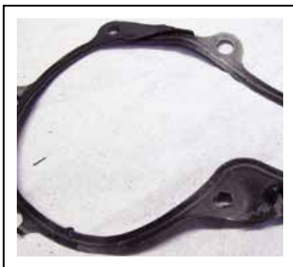
10.11 Sealant paste incorrectly applied on metal gasket
