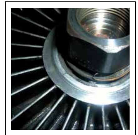
10.5 Damaged viscous coupling unit
