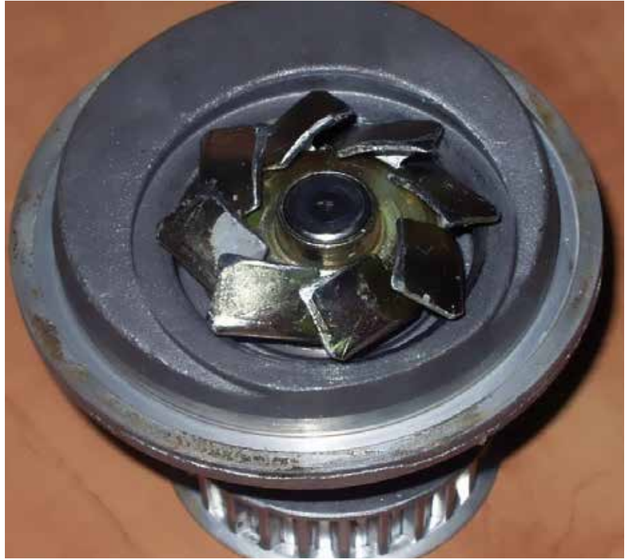
10.15 Impeller damaged by foreign object in the circuit
