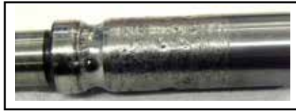
10.8 Bearing shaft damaged by excessive load
