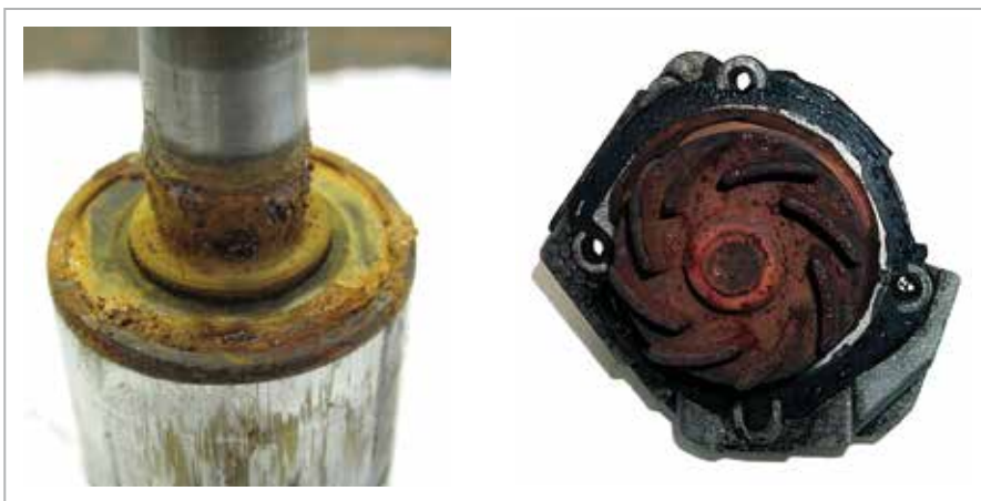
10.1 Rusted components due to unsuitable coolants
