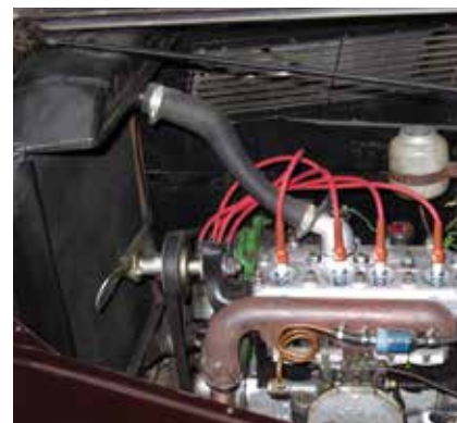
1.3 Old engine without water pump
