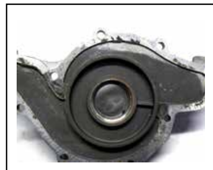
10.3 Sign of operation with air trapped inside
