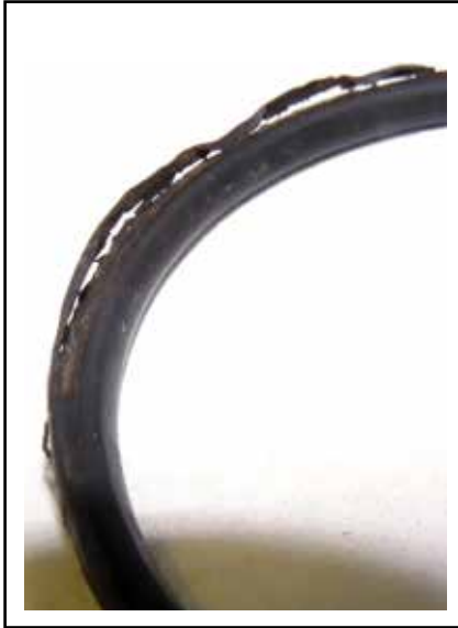
10.13 Damage caused by incorrect installation
