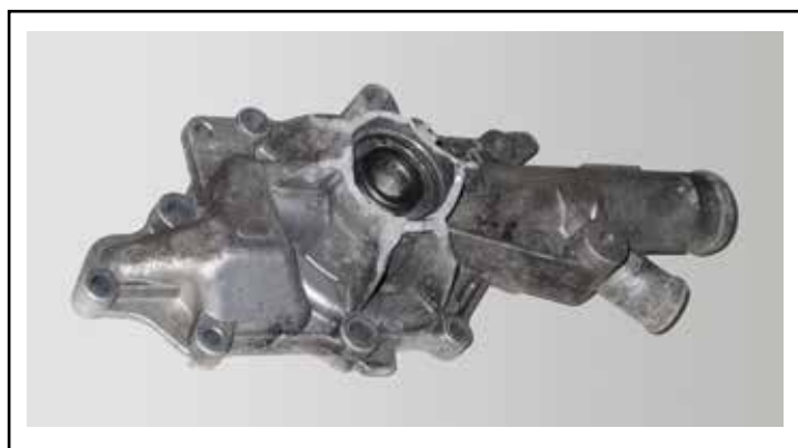
10.6 Complete failure of the pump casing due to unbalanced masses
