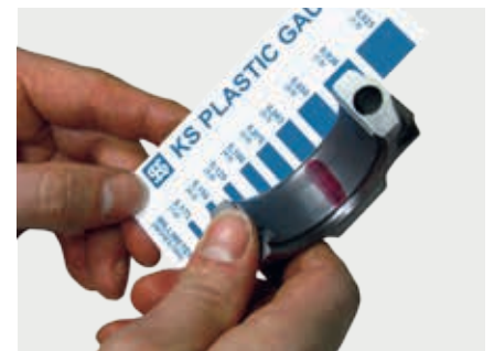
Checking the plain bearing with “KS Plastic Gauge”
