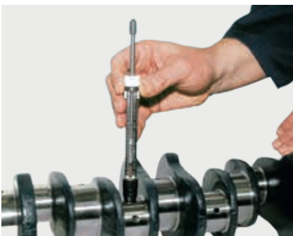
Hardness test with rebound hardness tester (item no. 50 009 812)
