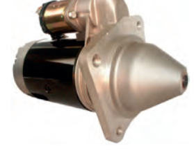
113381 Starter 12 V, 2.5 kW Replacing: AZJ3462, AZJ3195, AZJ3145, 11.139.456, 11.130.618, 11.130.510 Servicing: Farymann, Fiat, Fiat-Allis, Goldoni B+ M10, B- M8, Total length 340.00, Drive type Steel, Gear type DD, Mount. holes 3 (0) A: 109.70 B: 26.00 mm
