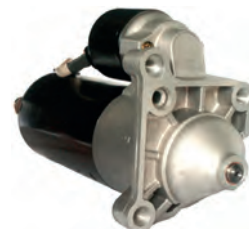
112295 Starter 12 V, 1.7 kW Replacing: D9RP256, D9R112, D7R5, D7R35, D7R25, D7R18, D7R13, D6RA112, D10E922, D10E921, D10E92, D10E85 Servicing: Mitsubishi, Renault, Volvo B+ M8, Total length 265.00, Drive type Steel, Gear type GR, Clutch type Dry, Mount. holes 3 (3) A: 66.00 B: -0.50 mm
