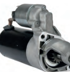
114850 Starter 12 V, 2.5 kW Replacing: 0001139409, 0001139408, 0001139030, 0001139029 Servicing: Mercedes-Benz B+ M8, Total length 240.00, Gear type GR, Mount. holes 2 (2) A: 70.00 B: 16.00 mm
