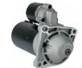
113430 Starter 12 V, 1.8 kW Replacing: AZE2111, 11.130.997 Servicing: Alfa Romeo, Fiat, Lancia, Suzuki B+ M8, Total length 226.00, Drive type Steel, Gear type GR, Mount. holes 3 (0) A: 81.50 B: 9.50 mm
