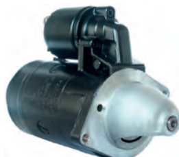
110793 Starter 12 V, 0.9 kW Replacing: 0001208211 Servicing: Citroen, Fiat, Peugeot B+ M8, Total length 221.00, Drive type Steel, Gear type DD, Mount. holes 2 (2) A: 66.00 B: 22.00 mm
