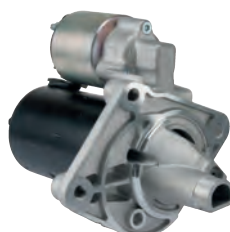
114294 Starter 12 V, 1.1 kW Replacing: 0001107064 Servicing: Chrysler, Plymouth B+ M8, Total length 239.00, Drive type Steel, Gear type GR, Mount. holes 3 (2) A: 70.00 B: 7.00 mm
