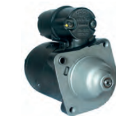
112289 Starter 12 V, 0.8 kW Replacing: D9E243, D9E123 Servicing: Fiat, Innocenti, Lancia B+ M8, 15a M5, Total length 224.00, Drive type Steel, Gear type DD, Mount. holes 3 (3) A: 64.20 B: 13.00 mm
