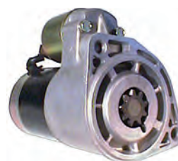
111549 Starter 12 V, 1.4 kW Replacing: S114-827, S114-762B, S114-762A, S114-762, S114-705E, S114-705D, S114-705C, S114-705B, S114-705A Servicing: Nissan B+ M8, Total length 199.00, Drive type Steel, Gear type GR, Mount. holes 2 (2) A: 82.45 B: 3.65 mm
