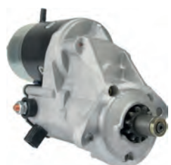
114711 Starter 12 V, 2.5 kW Replacing: 028000-7803, 028000-7802, 028000-7801, 028000-7800 Servicing: Kubota B+ M10, Total length 300.00, Gear type GR, Mount. holes 2 (0) A: 82.50 B: 25.00 mm
