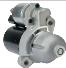
114837 Starter 12 V, 1.2 kW Replacing: 0001108406, 0001108405 Servicing: Audi B+ M8, Total length 213.50, Gear type GR, Mount. holes 2 (2) A: 66.00 B: 25.50 mm
