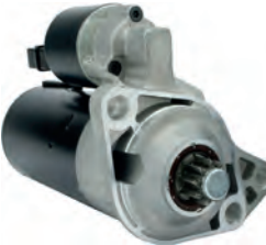
112286 Starter 12 V, 1.7 kW Replacing: 915109E, 9141396, 9141395, 443115141395 Servicing: Audi, Ford, Mercedes-Benz, Seat, Skoda, VW B+ M8, Total length 236.00, Drive type Steel, Gear type GR, Mount. holes 3 (0) A: 76.10 B: 32.00 mm
