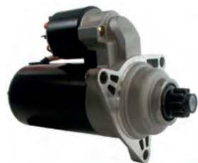
113387 Starter 12 V, 2.0 kW Replacing: AZE2625, 11.131.056 Servicing: Seat, VW B+ M8, Total length 238.00, Drive type Steel, Gear type GR, Mount. holes 3 (0) A: 76.00 B: 54.00 mm
