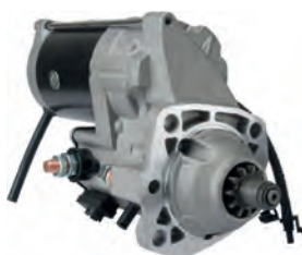
114712 Starter 24 V, 7.5 kW Replacing: 228000-9151, 228000-9150 Servicing: John Deere B+ M12, 30h Plug, Total length 316.00, Gear type GR, Mount. holes 3 (0) A: 88.80 B: 47.50 mm
