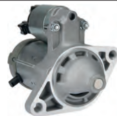
114886 Starter 12 V, 1.2 kW Replacing: 0001107449, 0001107448 Servicing: Toyota B+ M8, Total length 189.00, Gear type GR, Mount. holes 2 (1) A: 74.00 B: 14.00 mm
