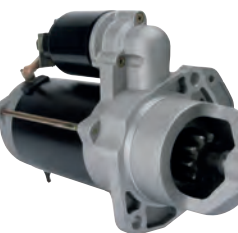
114307 Starter 24 V, 4.0 kW Replacing: 0001263024, 0001263023, 0001251004, 0001251003, 0001231039 Servicing: Case, Iveco B+ M10, Total length 314.00, Drive type Steel, Gear type GR, Mount. holes 3 (0) A: 89.00 B: 47.00 mm
