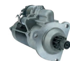
114527 Starter 24 V, 6.0 kW Replacing: 0001330004 Servicing: Volvo Penta B+ M10, B- M10, Total length 360.00, Drive type Steel, Gear type GR, Mount. holes 3 (0), Insulated return A: 92.00 B: 48.00 mm
