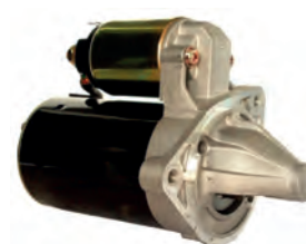
112322 Starter 12 V, 0.8 kW Replacing: TM000A37001, TM000A31001, M56290, 1195248 Servicing: Hyundai, Kia B+ M8, Total length 187.50, Drive type Steel, Gear type DD, Clutch type Dry, Mount. holes 2 (2) A: 75.00 B: 14.00 mm
