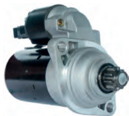
112005 Starter 12 V, 1.1 kW Replacing: 915111D Servicing: Audi, Seat, Skoda, VW B+ M8, Total length 211.50, Drive type Steel, Gear type GR, Clutch type Wet, Mount. holes 2 (0) A: 76.00 B: 52.00 mm
