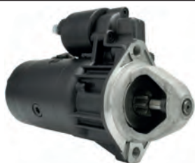
111120 Starter 12 V, 2.2 kW Replacing: S13-91A, S13-91 Servicing: Volvo, VW B+ M8, Total length 272.65, Drive type Steel, Gear type GR, Mount. holes 2 (2) A: 82.35 B: 21.60 mm
