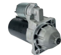
114402 Starter 12 V, 2.3 kW Replacing: 0001223022, 0001109356, 0001109355 Servicing: Mercruiser, Mercury, VM (Stabilimenti Mec) B+ M8x1.25, Total length 257.00, Drive type Steel, Gear type GR, Mount. holes 2 (0) A: 82.50 B: 16.00 mm
