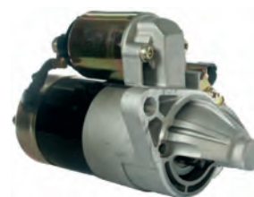
111459 Starter 12 V, 1.2 kW Replacing: S114-802A, S114-800C, S114-800B, S114-800A, S114-800, S114-767, S114-766A, S114-766, S114-750 Servicing: Jaguar, Nissan B+ M8, Total length 207.00, Drive type Steel, Gear type GR, Mount. holes 2 (1) A: 69.90 B: 11.50 mm
