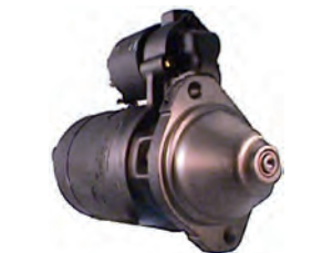
110838 Starter 12 V, 1.5 kW Replacing: B001315183, 0001315183, 0001314030, 0001314029, 0001314005 Servicing: Mercedes-Benz B+ M8, 15a M5, Total length 270.65, Drive type Steel, Gear type DD, Mount. holes 2 (2) A: 82.40 B: 20.25 mm
