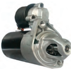
113282 Starter 12 V, 1.4 kW Manufacturer: Bosch Replacing: AZE2199, 11.139.431 Servicing: Chrysler, Mercedes-Benz B+ M8, Drive type Steel, Gear type GR, Mount. holes 2 (0) A: 60.00 B: 25.80 mm
