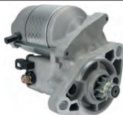
114718 Starter 12 V, 1.4 kW Replacing: 428000-3570 Servicing: Caterpillar, Perkins B+ M8, Total length 188.00, Gear type GR, Mount. holes 2 (0) A: 74.00 B: 19.00 mm
