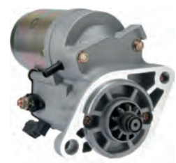
114731 Starter 12 V, 2.2 kW Replacing: 428000-2321 Servicing: Toyota B+ M8, Total length 235.00, Drive type Steel, Gear type GR, Mount. holes 2 (1) A: 82.50 B: 18.00 mm
