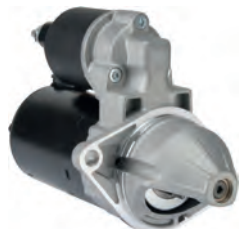
113276 Starter 12 V, 1.1 kW Replacing: AZD2126, 11.131.903 Servicing: Fiat, Mercedes-Benz, Opel, Saab, Vauxhall B+ M8, Total length 200.00, Drive type Steel, Gear type GR, Mount. holes 2 (0) A: 67.90 B: 19.00 mm
