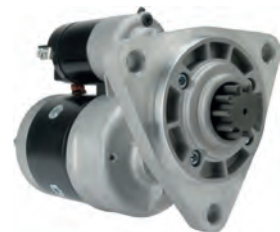
112488 Starter 12 V, 2.7 kW Replacing: 9142780, 443115142780 Servicing: Belarus B+ M10, Total length 238.50, Drive type Steel, Gear type GR, Clutch type Wet, Mount. holes 3 (0) A: 100.00 B: 32.00 mm
