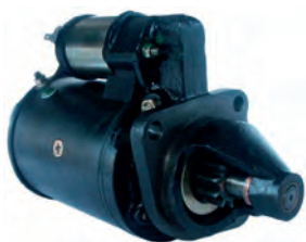
110615 Starter 12 V, 2.8 kW Replacing: 9004475035 Servicing: Agco Allis, Agco White, Allis Chalmers, Atlas Copco, JCB, Massey Ferguson, Perkins B+ M8, Total length 312.25, Drive type Steel, Gear type DD, Mount. holes 3 (0) A: 89.00 B: 28.60 mm
