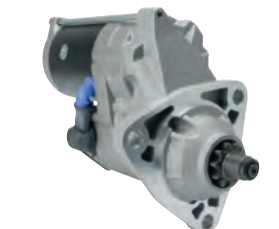
113429 Starter 12 V, 4.2 kW Replacing: AZF4611, AZF4577, 11.131.300, 11.131.117 Servicing: Case, Cummins B+ M10, B- M12, Total length 317.00, Drive type Steel, Gear type GR, Mount. holes 3 (0) A: 92.00 B: 47.50 mm
