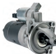
114304 Starter 12 V, 2.3 kW Replacing: 6033AB1J00, 0001218822, 0001109417 Servicing: VW B+ M8, Total length 272.00, Drive type Steel, Gear type GR, Clutch type Dry, Mount. holes 3 (0) A: 110.00 B: 27.00 mm
