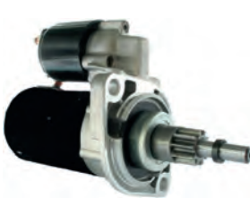
112131 Starter 12 V, 1.4 kW Replacing: 9141410 Servicing: VW B+ M8, 15a 6.30, Total length 244.00, Drive type Steel, Gear type GR, Mount. holes 2 (0) Bushing D.E. (clutch house): HC-CARGO 140018. A: 76.00 B: 52.00 mm
