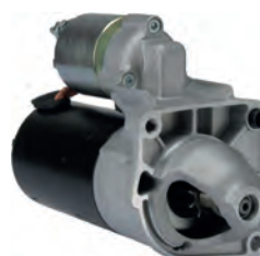
115312 Starter 12 V, 1.1 kW Replacing: 0001170403, 0001170402, 0001170401, 0001137012, 0001137011, 0001137002, 0001137001 Servicing: Alfa Romeo, Fiat, Ford, Lancia B+ M8, Total length 218.00, Gear type GR, Mount. holes 3 (1) A: 64.00 B: 10.50 mm
