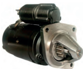
112074 Starter 12 V, 3.1 kW Replacing: 9142766 Servicing: Ford, New Holland B+ M8, Total length 329.00, Drive type Steel, Gear type DD, Mount. holes 3 (0) A: 92.00 B: 21.00 mm
