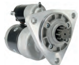
113356 Starter 24 V, 3.5 kW Replacing: AZJ3223, 11.130.676 Servicing: Belarus, GAZ, ZIL B+ M10, Total length 235.00, Drive type Steel, Gear type GR, Mount. holes 3 (0) A: 99.90 B: 32.00 mm
