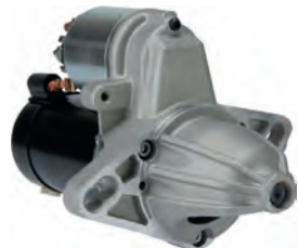
112217 Starter 12 V, 1.0 kW Replacing: D6RA80, D6RA67, D6RA167 Servicing: Honda, Rover B+ M8, Drive type Steel, Gear type GR, Mount. holes 2 (0) A: 75.00 B: 33.50 mm
