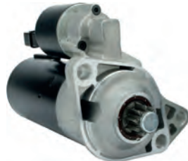
112286 Starter 12 V, 1.7 kW Replacing: D7RS29, D7RS129 Servicing: Audi, Ford, Mercedes-Benz, Seat, Skoda, VW B+ M8, Total length 236.00, Drive type Steel, Gear type GR, Mount. holes 3 (0) A: 76.10 B: 32.00 mm
