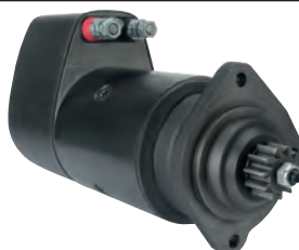
114438 Starter 24 V, 5.4 kW Replacing: 0001416032 Servicing: KHD, Liebherr, Orenstein and koppel B+ M10, B- M10, Mount. holes 3 (0), Insulated return A: 89.00 B: 47.50 mm
