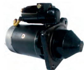
110640 Starter 12 V, 3.0 kW Replacing: 0001367014, 0001359091 Servicing: Allis Chalmers, Fiat, Fiat-Allis, Long B+ M10, Total length 310.00, Drive type Steel, Gear type DD, Mount. holes 3 (0) A: 110.00 B: 26.00 mm
