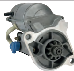
114748 Starter 12 V, 1.4 kW Replacing: 128000-5590 Servicing: Case B+ M8, 15a M4, Total length 189.00, Gear type GR, Mount. holes 2 (0) A: 89.00 B: 20.00 mm
