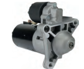
113443 Starter 12 V, 1.4 kW Replacing: AZE2534, 11.130.716 Servicing: Citroen, Fiat, Peugeot B+ M8, Total length 240.00, Drive type Steel, Gear type GR, Mount. holes 3 (3) A: 62.10 B: -5.00 mm
