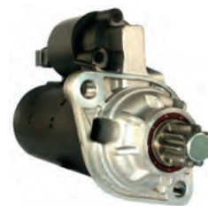
112429 Starter 12 V, 2.0 kW Replacing: 915109D Servicing: Audi, Ford, Seat, Skoda, VW B+ M8, Total length 259.00, Drive type Steel, Gear type GR, Mount. holes 2 (0) A: 76.00 B: 62.00 mm
