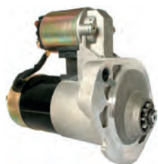
111136 Starter 12 V, 1.4 kW Replacing: S114-480B, S114-480A, S114-480, S114-473 Servicing: Opel, Vauxhall B+ M8, Total length 199.00, Drive type Steel, Gear type GR, Mount. holes 2 (1) A: 77.90 B: 19.00 mm
