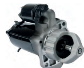
114523 Starter 24 V, 4.0 kW Replacing: B001260015, 0001263049, 0001263016, 0001263015, 0001231133, 0001231033, 0001231032, 0001231002 Servicing: Mercedes-Benz B+ M10, Total length 313.00, Drive type Steel, Gear type GR, Mount. holes 3 (0) Alternative no.: 115514 A: 89.00 B: 48.50 mm
