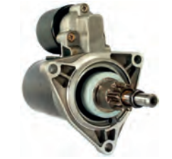
112306 Starter 12 V, 1.1 kW Replacing: 9141390 Servicing: VW B+ M8, Total length 254.00, Drive type Steel, Gear type GR, Clutch type Dry, Mount. holes 3 (0) Bushing D.E. (clutch house): HC-CARGO 140018. A: 76.00 B: 52.00 mm
