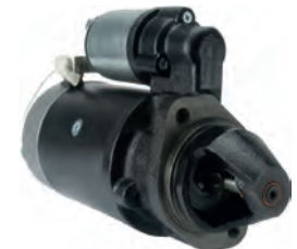
110775 Starter 12 V, 1.8 kW Replacing: 0001362038, 0001362028, 0001362027, 0001362004, 0001362003 Servicing: Claas, Mercedes-Benz B+ M10, Total length 288.00, Drive type Steel, Gear type DD, Clutch type Wet, Mount. holes 2 (0) A: 83.00 B: 20.00 mm
