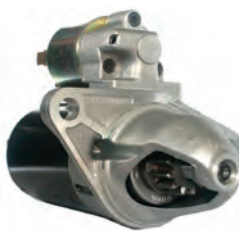
113281 Starter 12 V, 1.1 kW Replacing: AZE2211, 11.139.448 Servicing: MG, Rover B+ M8, Total length 231.40, Drive type Steel, Gear type GR, Clutch type Dry, Mount. holes 2 (0) A: 75.00 B: 43.00 mm
