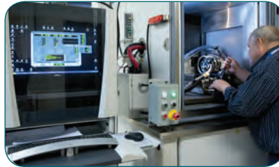
Alternator duration test
