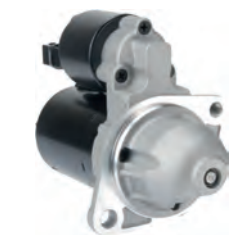
114740 Starter 12 V, 1.2 kW Replacing: 428000-4490, 428000-1760 Servicing: BMW B+ M8, Total length 222.00, Gear type GR, Mount. holes 2 (1) A: 76.00 B: 25.00 mm
