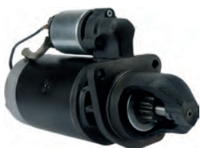
114397 Starter 24 V, 4.0 kW Replacing: 0001368067 Servicing: Cummins B+ M10, Total length 340.00, Drive type Steel, Gear type DD, Mount. holes 3 (0), Insulated return A: 89.00 B: 48.20 mm
