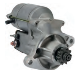
114738 Starter 12 V, 1.4 kW Replacing: 228000-6652, 228000-6651, 228000-6650 Servicing: Bobcat B+ M8, Total length 218.00, Gear type GR, Mount. holes 2 (0) A: 88.80 B: 48.00 mm
