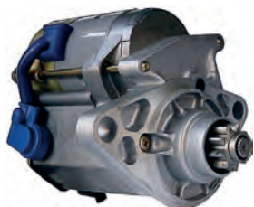
112214 Starter 12 V, 1.6 kW Replacing: D7RSA5, D7RSA4, D7RSA11, D7RSA10 Servicing: Honda, Rover B+ M8, Total length 210.00, Drive type Steel, Gear type GR, Mount. holes 2 (0) A: 75.00 B: 40.00 mm
