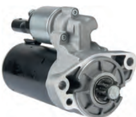
114775 Starter 12 V, 2.2 kW Replacing: 0001125610, 0001125609 Servicing: Audi, VW B+ M8, Total length 235.50, Drive type Steel, Gear type GR, Mount. holes 3 (1) Alternative no.: 115502 A: 76.20 B: 25.00 mm
