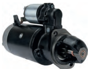
114398 Starter 24 V, 4.0 kW Replacing: 0001368071, 0001368050, 0001368046 Servicing: Hatz B+ M10, Total length 345.00, Gear type DD, Mount. holes 2 (0) A: 82.50 B: 21.00 mm
