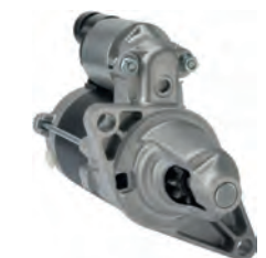
114816 Starter 12 V, 0.8 kW Replacing: 228000-9580 Servicing: Honda B+ M8, Total length 205.00, Gear type DD, Mount. holes 2 (0) A: 75.00 B: 33.50 mm
