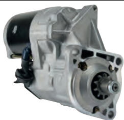
114695 Starter 24 V, 7.5 kW Replacing: 428000-2591, 428000-2590 Servicing: Case B+ M12, Total length 317.00, Gear type GR, Mount. holes 3 (0) A: 88.88 B: 28.00 mm
