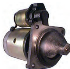
110812 Starter 12 V, 2.0 kW Replacing: 0001362073 Servicing: Alfa Romeo, Fiat, Seat B+ M10, Total length 293.00, Drive type Steel, Gear type DD, Clutch type Dry, Mount. holes 3 (0) A: 110.00 B: 27.00 mm
