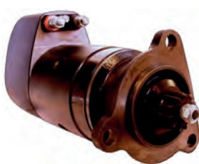
112119 Starter 24 V, 6.6 kW Replacing: 9125110 Servicing: Scania B+ M10, B- M10, Total length 406.00, Drive type Steel, Gear type DD, Mount. holes 3 (0) A: 92.00 B: 37.00 mm
