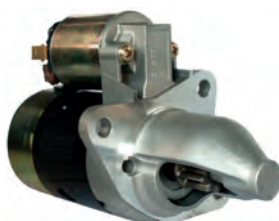
113346 Starter 12 V, 0.8 kW Replacing: AZJ3281, 11.130.783 Servicing: MG, Rover, VW B+ M8, Total length 210.50, Drive type Steel, Gear type DD/GR, Mount. holes 3 (0) A: 67.00 B: 39.50 mm
