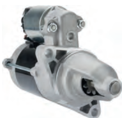
114716 Starter 12 V Replacing: 428000-0230 Servicing: Briggs & Stratton B+ M8, Total length 208.00, Gear type DD, Mount. holes 2 (0) A: 70.00 B: 32.50 mm
