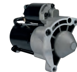
114460 Starter 12 V, 1.4 kW Replacing: 0001108400, 0001108183 Servicing: Citroen, Fiat, Hyundai, Lancia, Mitsubishi, Peugeot B+ M8, Total length 216.00, Gear type GR, Mount. holes 3 (3) B: -4.00 mm
