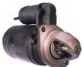
110772 Starter 12 V, 1.0 kW Replacing: 0001311045, 0001311025, 0001311016 Servicing: BMW B+ M8, 15a 6.30, Total length 271.25, Drive type Steel, Gear type DD, Clutch type Dry, Mount. holes 2 (0) A: 76.00 B: 27.30 mm
