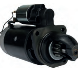
114266 Starter 24 V, 4.0 kW Replacing: 0001368015 Servicing: Agco Power (Sisu Diesel) B+ M10, B- M8, Total length 346.50, Gear type DD, Mount. holes 3 (0), Insulated return A: 89.00 B: 48.00 mm
