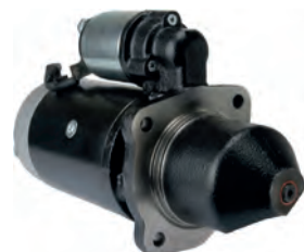
112442 Starter 12 V, 3.0 kW Replacing: 9142745 Servicing: John Deere B+ M10, Total length 340.00, Drive type Steel, Gear type DD, Clutch type Dry, Mount. holes 3 (0) GR Starter HC-CARGO 115609. A: 89.00 B: 48.00 mm
