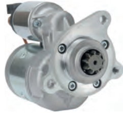
112388 Starter 12 V, 1.0 kW Replacing: 9141331, 443115141338, 443115141331 Servicing: Skoda B+ M8, Total length 199.00, Drive type Steel, Gear type GR, Clutch type Wet, Mount. holes 3 (1) A: 50.00 B: 21.00 mm
