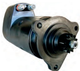
112116 Starter 24 V, 6.6 kW Replacing: FS60PR171 Servicing: Volvo B+ M12, B- M12, Total length 407.00, Drive type Steel, Gear type DD, Mount. holes 3 (0), Insulated return A: 92.00 B: 47.00 mm
