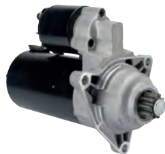
112167 Starter 12 V, 1.8 kW Replacing: 9141319 Servicing: VW B+ M8, Total length 236.00, Drive type Steel, Gear type GR, Mount. holes 3 (0) Bushing D.E. (clutch house): HC-CARGO 140018. A: 76.00 B: 52.00 mm
