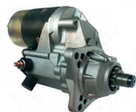
112822 Starter 24 V, 4.5 kW Replacing: 9122110 Servicing: Iveco B+ M10, Total length 293.00, Drive type Steel, Gear type GR, Clutch type Wet, Mount. holes 3 (0) Alternative no.: 115880 A: 89.00 B: 49.00 mm
