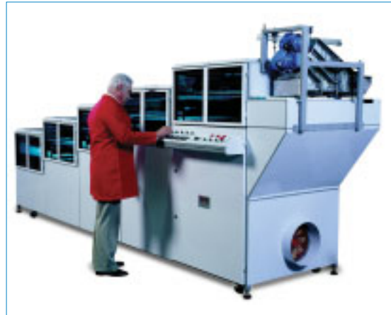
■ Fig 19. UV “cascade” surface disinfection of spices.
