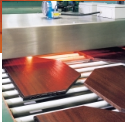
Coating of wood parts
