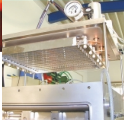
Vacuum plant with infrared emitters
