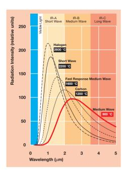
Spectrum of the medium wave infrared emitter compared with other Heraeus infrared emitters – taken at the same electrical power for all emitter types.
