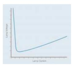
The provision of a main power supply to the first intersection, where the lamp is driven by the trigger pulse, is generally uneconomic (it requires a much higher voltage than is needed for running). The usual solution is to have a boost power supply with the load line indicated by the line XY. As it is only required at start up, the supply can be fairly low cost. Usually a small low current power supply charges up a capacitor; the capacitor acting as a very short duration power supply.
