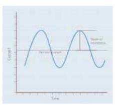
Fig.26 Modulated CW operation
