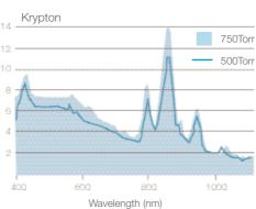
The dominant radiation emission mechanism in Krypton filled CW lamps is through bound-bound transitions. This gives rise to a line spectrum in the infrared region (figure 14) which satisfactorily overlaps the absorption bands of Nd:YAG.
