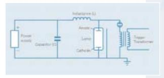
Fig.22 Typical external triggering circuit
