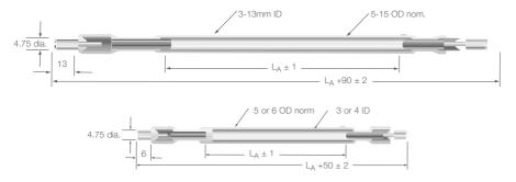
Fig.37 Air-cooled pulse lamp recommended physical dimensions (mm)
