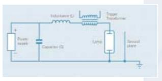
Fig.21 Typical parallel triggering circuit
