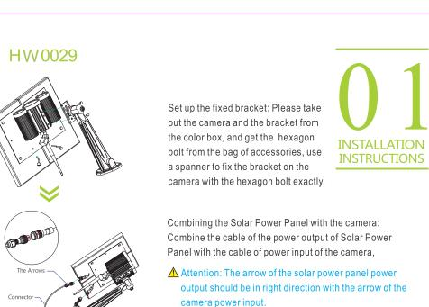
Combining the Solar Power Panel with the camera: Combine the cable of the power output of Solar Power Panel with the cable of power input of the camera, 1 Attention: The arrow of the solar power panel power output should be in right direction with the arrow of the camera power input.
