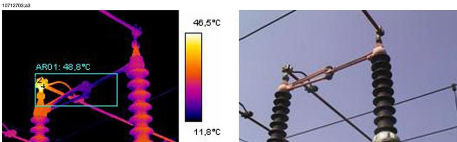
**Figure 25.1** An infrared and a visual image of a power line isolator
