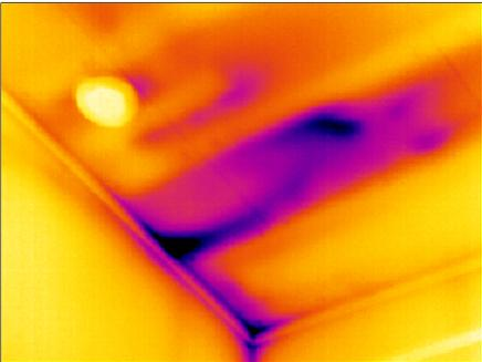
An infrared thermography image of a floor structure. The image shows a dark, irregular shape in the center, which is a sign of insulation deficiencies. The surrounding areas are lighter, indicating higher temperatures. The image is labeled '10553503.a1' in the top left corner. | <p data-bbox="571 164 1008 268">Insulation deficiencies in an intermediate floor structure. The deficiency may be due to either missing insulation batts or improperly installed insulations batts (air pockets).</p> |
