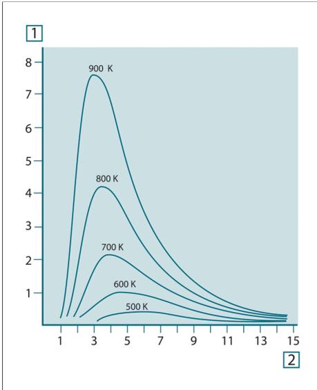
**Figure 30.4** Blackbody spectral radiant emittance according to Planck's law, plotted for various absolute temperatures. **1:** Spectral radiant emittance ( $\text{W}/\text{cm}^2 \times 10^3(\mu\text{m})$ ); **2:** Wavelength ( $\mu\text{m}$ )
