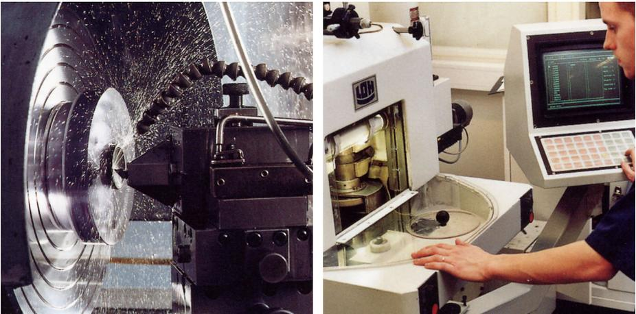
**Figure 26.3** LEFT: Diamond turning machine; RIGHT: Lens polishing
