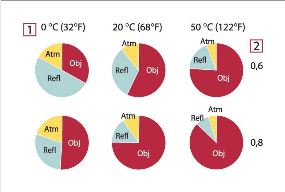
**Figure 31.3** Relative magnitudes of radiation sources under varying measurement conditions (SW camera). **1:** Object temperature; **2:** Emittance; **Obj:** Object radiation; **Refl:** Reflected radiation; **Atm:** atmosphere radiation. Fixed parameters:  $\tau = 0.88$ ;  $T_{\text{refl}} = 20^\circ\text{C}$  (+68°F);  $T_{\text{atm}} = 20^\circ\text{C}$  (+68°F).
