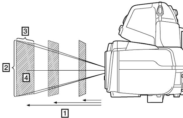
**Figure 21.2** Relationship between the field of view and distance. 1: Distance to target; 2: VFOV = vertical field of view; 3: HFOV = horizontal field of view, 4: IFOV = instantaneous field of view (size of one detector element).
