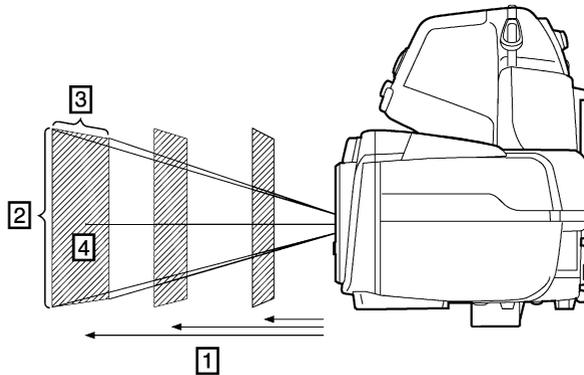
**Figure 21.4** Relationship between the field of view and distance. 1: Distance to target; 2: VFOV = vertical field of view; 3: HFOV = horizontal field of view, 4: IFOV = instantaneous field of view (size of one detector element).
