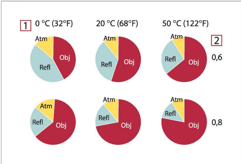
**Figure 31.4** Relative magnitudes of radiation sources under varying measurement conditions (LW camera). **1:** Object temperature; **2:** Emittance; **Obj:** Object radiation; **Refl:** Reflected radiation; **Atm:** atmosphere radiation. Fixed parameters:  $\tau = 0.88$ ;  $T_{\text{refl}} = 20^{\circ}\text{C}$  (+68°F);  $T_{\text{atm}} = 20^{\circ}\text{C}$  (+68°F).
