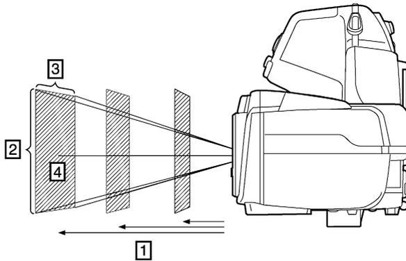
**Figure 21.3** Relationship between the field of view and distance. 1: Distance to target; 2: VFOV = vertical field of view; 3: HFOV = horizontal field of view, 4: IFOV = instantaneous field of view (size of one detector element).
