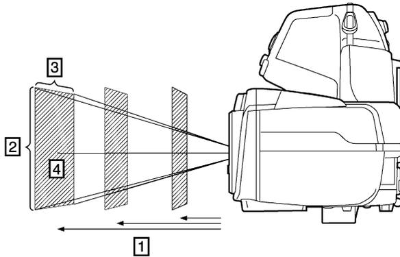
**Figure 21.5** Relationship between the field of view and distance. 1: Distance to target; 2: VFOV = vertical field of view; 3: HFOV = horizontal field of view, 4: IFOV = instantaneous field of view (size of one detector element).
