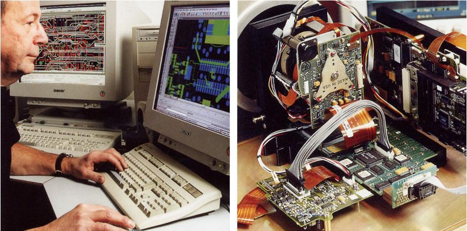
**Figure 26.2** LEFT: Development of system electronics; RIGHT: Testing of an FPA detector
