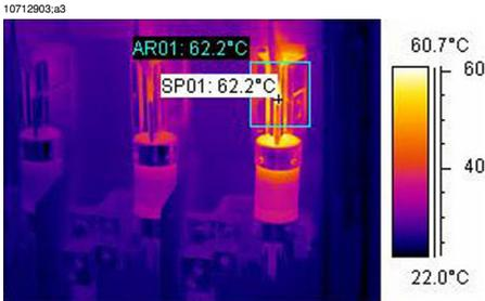
**Figure 25.3** An infrared image of a fusebox where the maximum temperature is displayed
