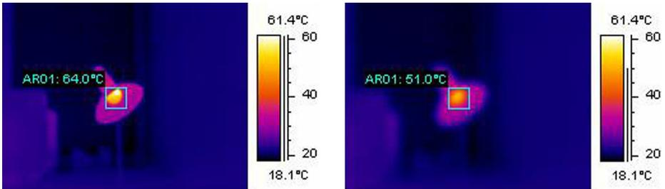
**Figure 25.5** LEFT: A hot spot in focus; RIGHT: A hot spot out of focus
