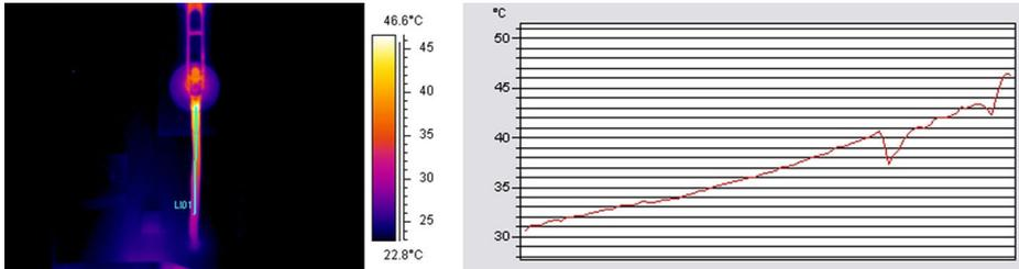
**Figure 25.7** A profile (line) in an infrared image and a graph displaying the increasing temperature
