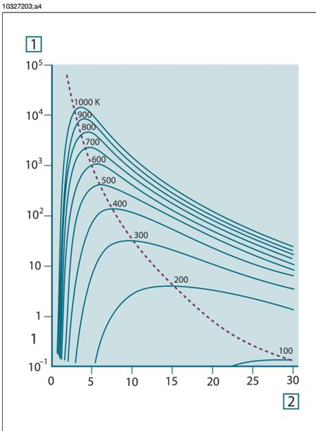
**Figure 30.6** Planckian curves plotted on semi-log scales from 100 K to 1000 K. The dotted line represents the locus of maximum radiant emittance at each temperature as described by Wien's displacement law. 1: Spectral radiant emittance ( $\text{W}/\text{cm}^2 (\mu\text{m})$ ); 2: Wavelength ( $\mu\text{m}$ ).
