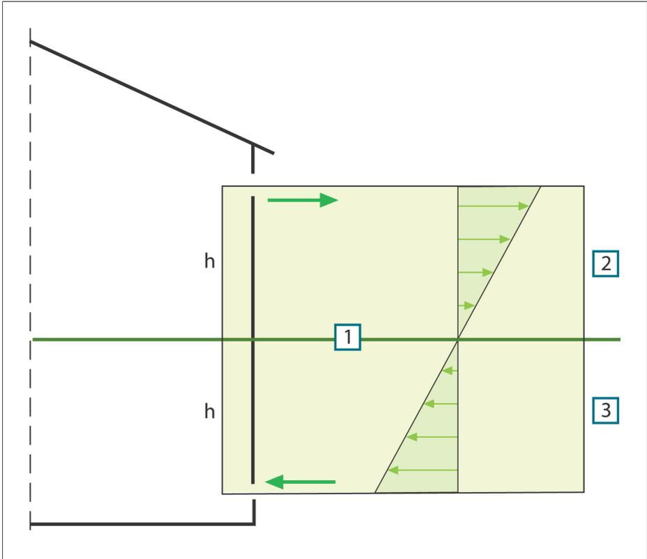
**Figure 24.5** Distribution of pressures on a building with two openings and where the external temperature is lower than the internal temperature. 1: Neutral zone; 2: Positive pressure; 3: Negative pressure; **h**: Distance from the neutral zone in meters.
