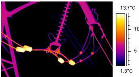
**Figure 25.13** An infrared image of hot stabilizing weights
