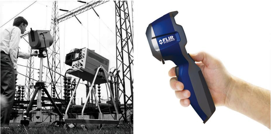
**Figure 26.1 LEFT:** Thermovision® Model 661 from 1969. The camera weighed approximately 25 kg (55 lb.), the oscilloscope 20 kg (44 lb.), and the tripod 15 kg (33 lb.). The operator also needed a 220 VAC generator set, and a 10 L (2.6 US gallon) jar with liquid nitrogen. To the left of the oscilloscope the Polaroid attachment (6 kg/13 lb.) can be seen. **RIGHT:** FLIR i5 from 2008. Weight: 0.34 kg (0.75 lb.), including the battery.
