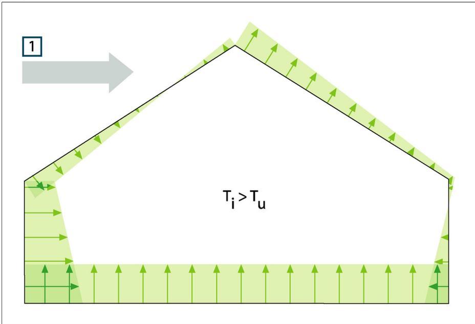
**Figure 24.3** Distribution of resultant pressures on a building's enclosing surfaces depending on wind effects, ventilation and internal/external temperature difference. 1: Wind direction;  $T_u$ : Thermodynamic air temperature outdoors in K;  $T_i$ : Thermodynamic air temperature indoors in K.
