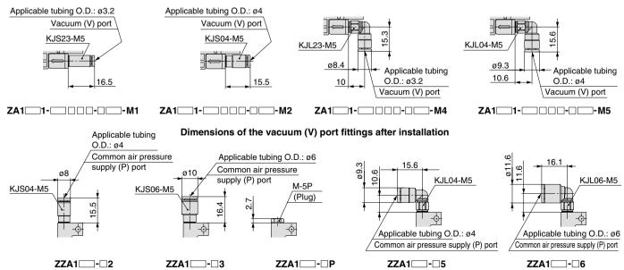
Dimensions after the fittings are installed on the common air pressure supply (P) port
