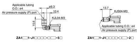
Dimensions of the air pressure supply (P) port fittings after installation
