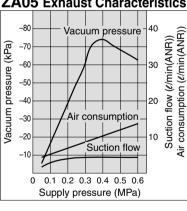
**ZA05** Flow Characteristics Supply pressure: 0.4 MPa -80 Vacuum pressure (kPa) -60 -40 -20 Suction flow (@min(ANR))
