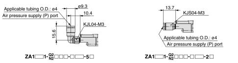
Dimensions of the air pressure supply (P) port fittings after installation
