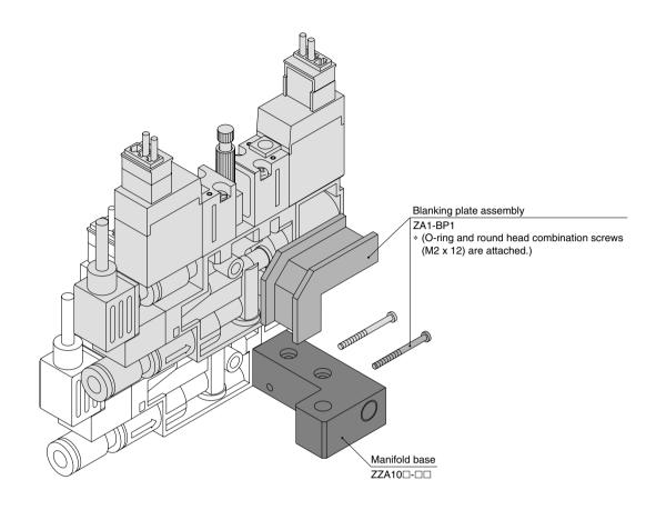
\* An assembly kit (part no. ZA1-OP-1) is available which includes 10 pcs each of O-rings and round head combination screws. ZA
