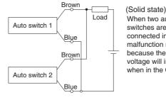
Load impedance = 1 mA x 2 pcs. x 3 k $\Omega$ = 6 V
