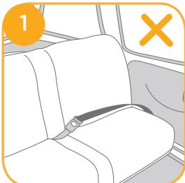
! This infant child restraint is suitable for vehicle seats with a 3-point Retractor Safety Belt (with or without base) ONLY ②, and ISOFIX anchor points WITH the Base. ③
