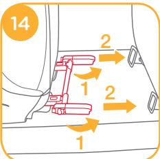
3. Line up the Isosafe connectors with the ISOFIX anchor points, and then click both Isosafe connectors into the ISOFIX anchor points. **15**
