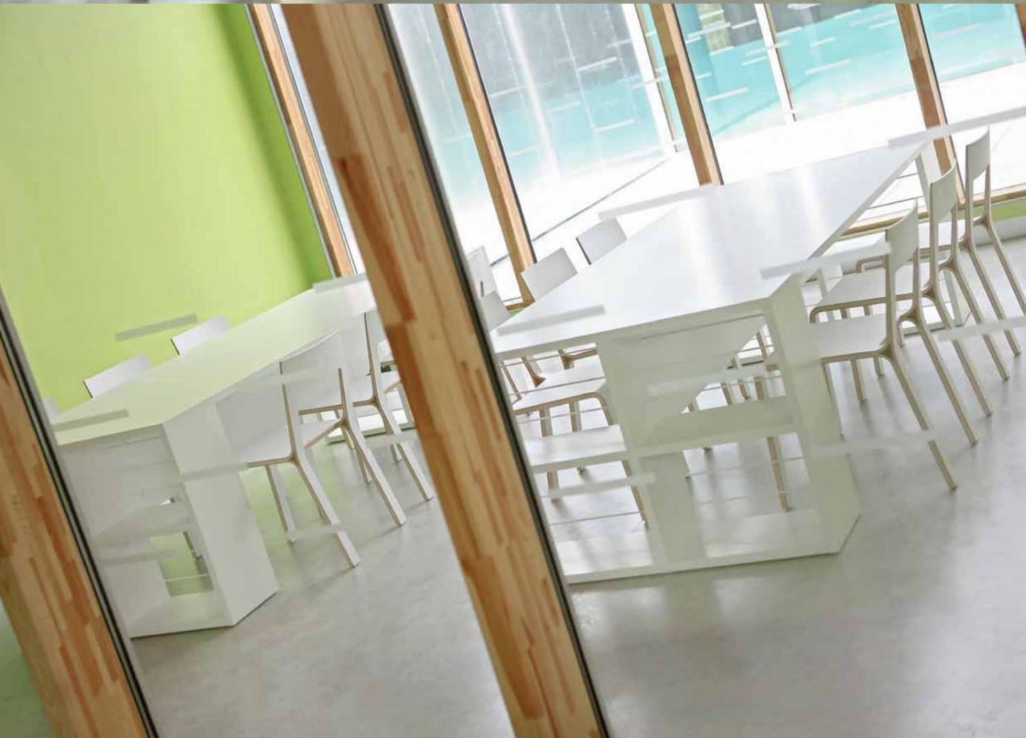
FRAME IS A MONO-BLOCK CHAIR, MOULDED IN ONE PIECE OF PLYWOOD WITH VARIABLE THICKNESS AND SOLID WOOD INSERT. THE WHOLE CHAIR IS PRESSED IN ONE SINGLE PROCESS. UNUSUAL SIDEWAYS STACKING IDEA ALLOWS THE CHAIR TO STACK AND KEEP A SIMPLE, CLEAR, ALMOST CLASSIC FORM – WELL PROPORTIONED AND ERGONOMIC. THE SQUARE CUT IN THE BACKREST GIVES THE FEELING OF TRANSPARENCY. PURE AND AESTHETIC DESIGN OF FRAME OFFERS POSITIVE EXPERIENCES FOR ARCHITECTS AND CUSTOMERS.
