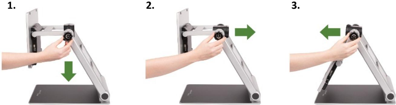
You can switch between modes by rotating/adjusting the camera using the Camera Positioning wheel.
