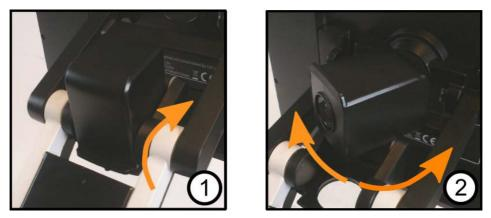
The camera has two modes. Reading mode and distance mode. Turn the camera to switch it from reading mode (1) to distance mode (2). When the camera is in distance mode, it can be angled laterally, depending on what you want to look at. In distance mode, the camera can also be turned to a mirror mode. The settings for both modes are automatically saved when you switch from one to the other.
