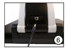
6. Connect the mains adapter to the rear of the unit and to the wall socket. The unit is now ready to be used.
