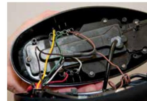
FIGURE 18 Insert AutoPilot wires into terminal holders.
