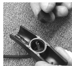
Remove the plug in the handle. Untie the knot in the rope. Slip the rope out of the handle.
