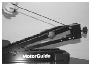
Raise Bow Arm to 45 Degree Angle
