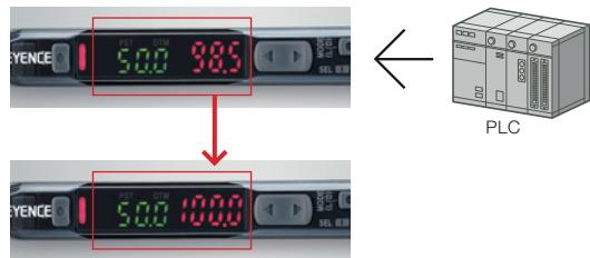
The sensor can be calibrated from a PLC or other external device. Regularly executing the Preset function from an external input ensures uninterrupted, stable detection, even in harsh environments. The 2-output type can be used to provide a low light intensity signal if the sensor becomes extremely dirty.
