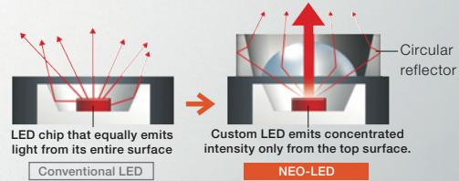
The circular reflector helps compensate for light positioning errors by redirecting any stray light back into the fiber.
