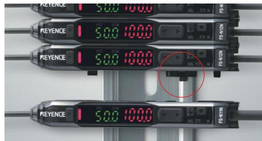
When adding sensors, the power is supplied from the connector on the side. This reduces wiring by two cables per sensor, allowing for a neater, quicker installation.
