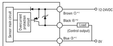
Input Circuit Diagram (FS-N13P/N14P only)
