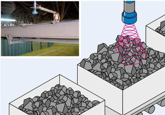
Regulating and monitoring the filling level of liquids and bulk materials ensures process reliability regardless of the material in question
