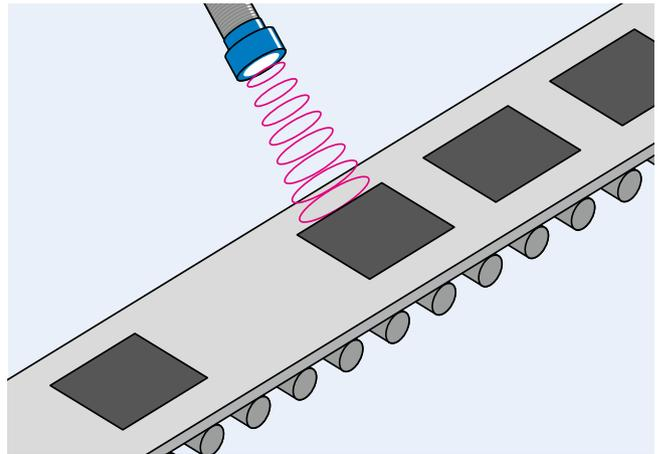
Detecting very flat objects which are difficult to detect optically using edge detection maximizes productivity
