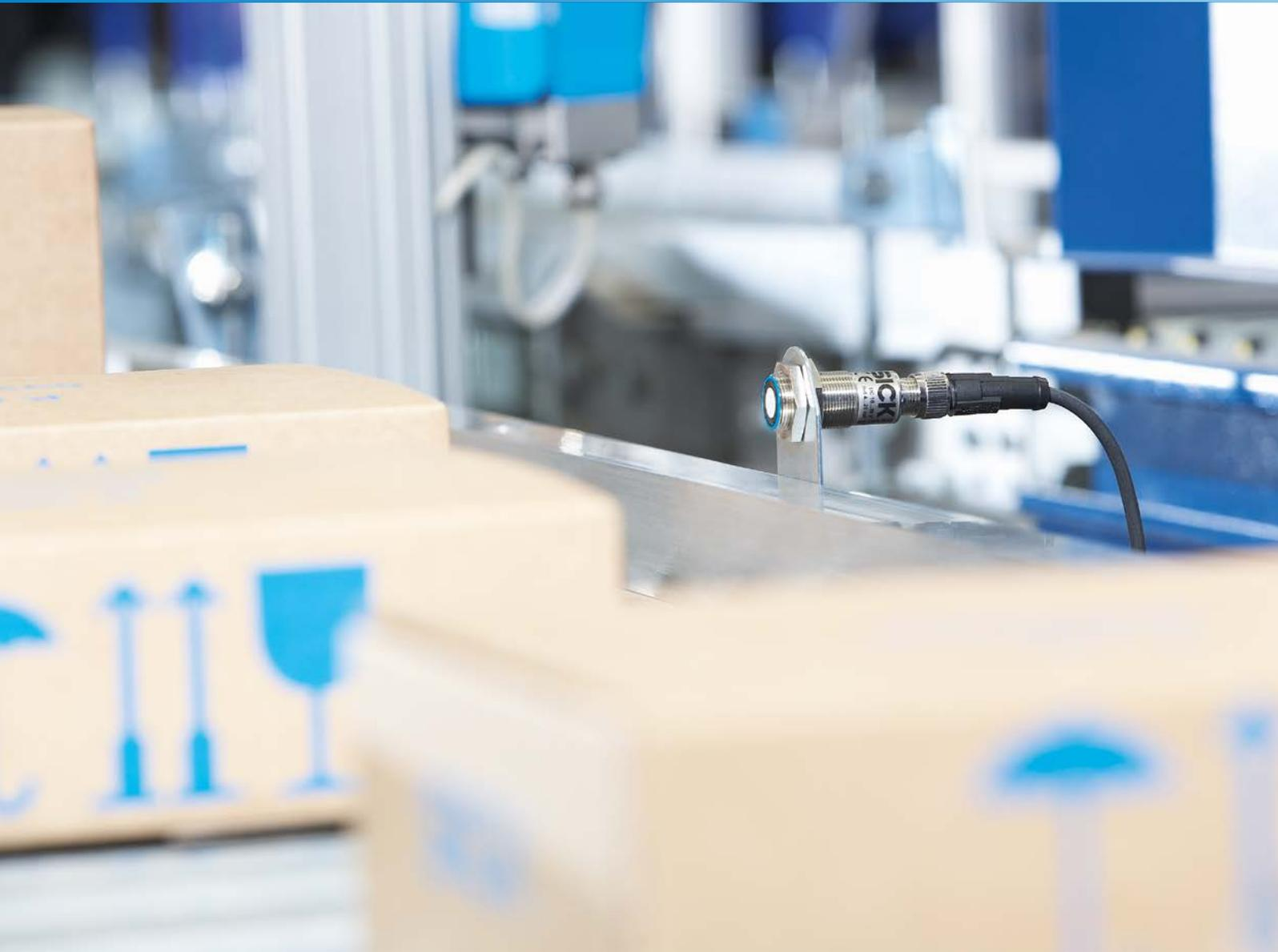
Ultrasonic sensors from SICK perform measurement and detection in a wide variety of application areas on colored, shiny, or transparent surfaces, which are particularly challenging for optical sensors. Even adverse ambient conditions such as dust, dirt, or fog hardly affect the measurement result. The broad detection range also allows for a large field to be monitored with just one sensor – with a measuring range of 13 mm to 8 m.
