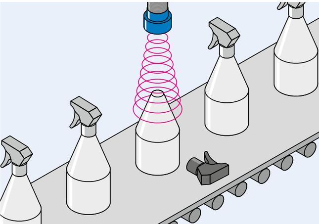
Detecting incorrectly produced or unfinished goods and incorrect alignment reduces system downtimes and ensures highest productivity
