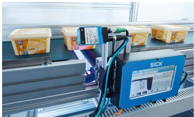
Quality control during the packaging process: The Inline Code Matcher ensures that the right product is in the right packaging.
