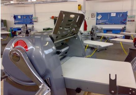
Safety guard open for replacing the scraper. In this case the machine can not working.
