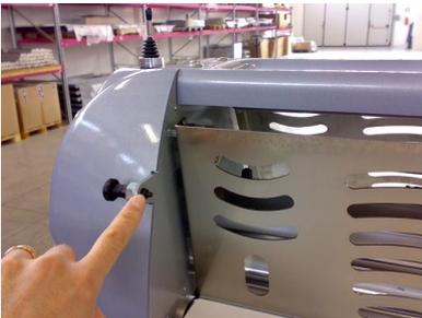
Pin for locking the tables when the tables are closed (Fig. 14)
