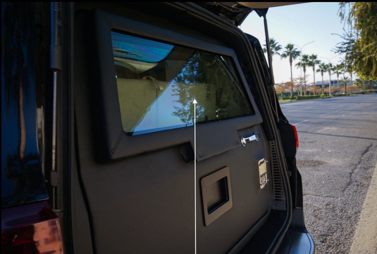
Ballistic barrier with a door and loophole with built-in laminated ballistic glass with an internal polycarbonate layer for protection against fragments inside and for an emergency exit in case of an armed attack or a traffic accident
