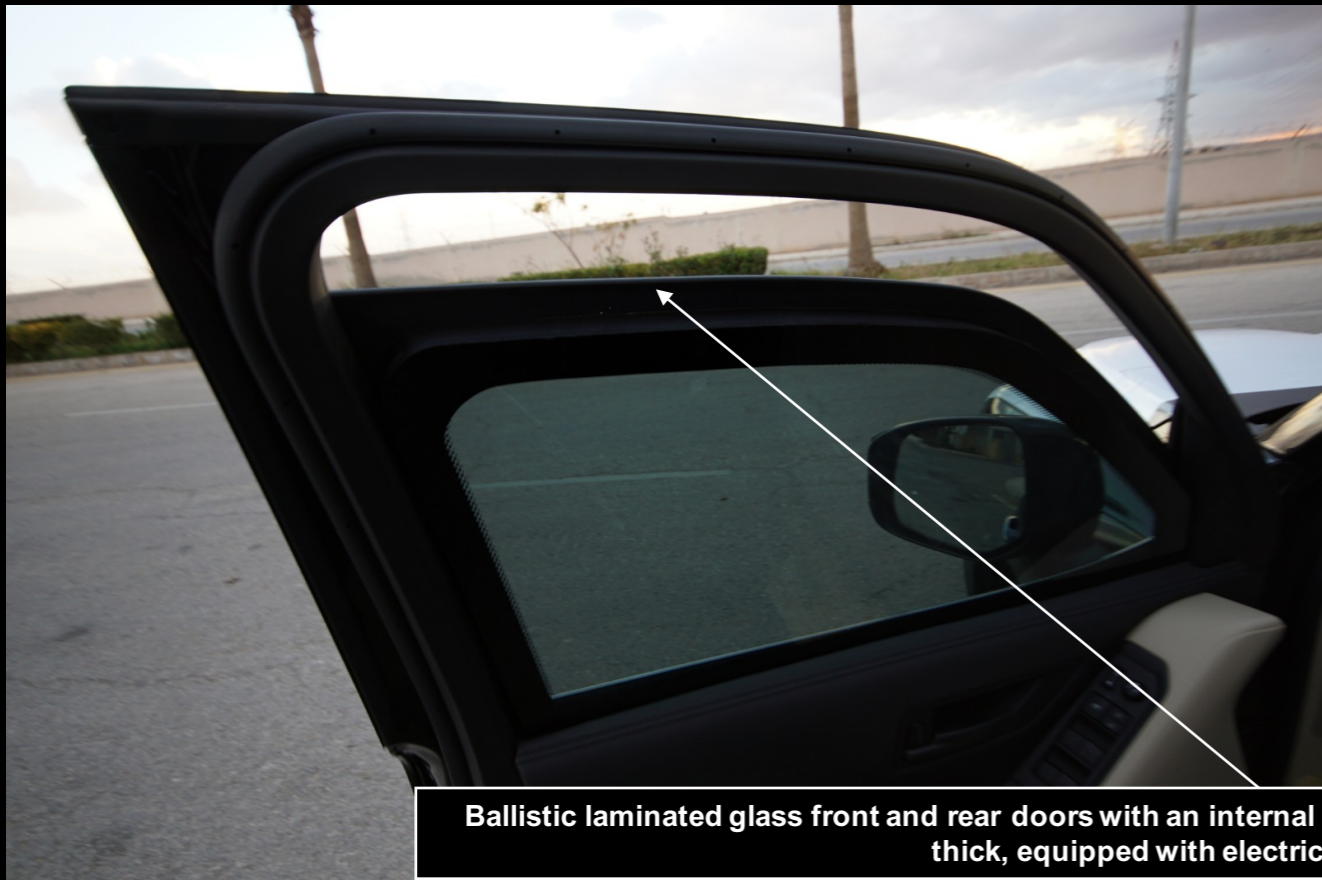
Overlapping overlapping of doorways from the penetration of bullets and shrapnel when firing firearms and detonating IEDs
