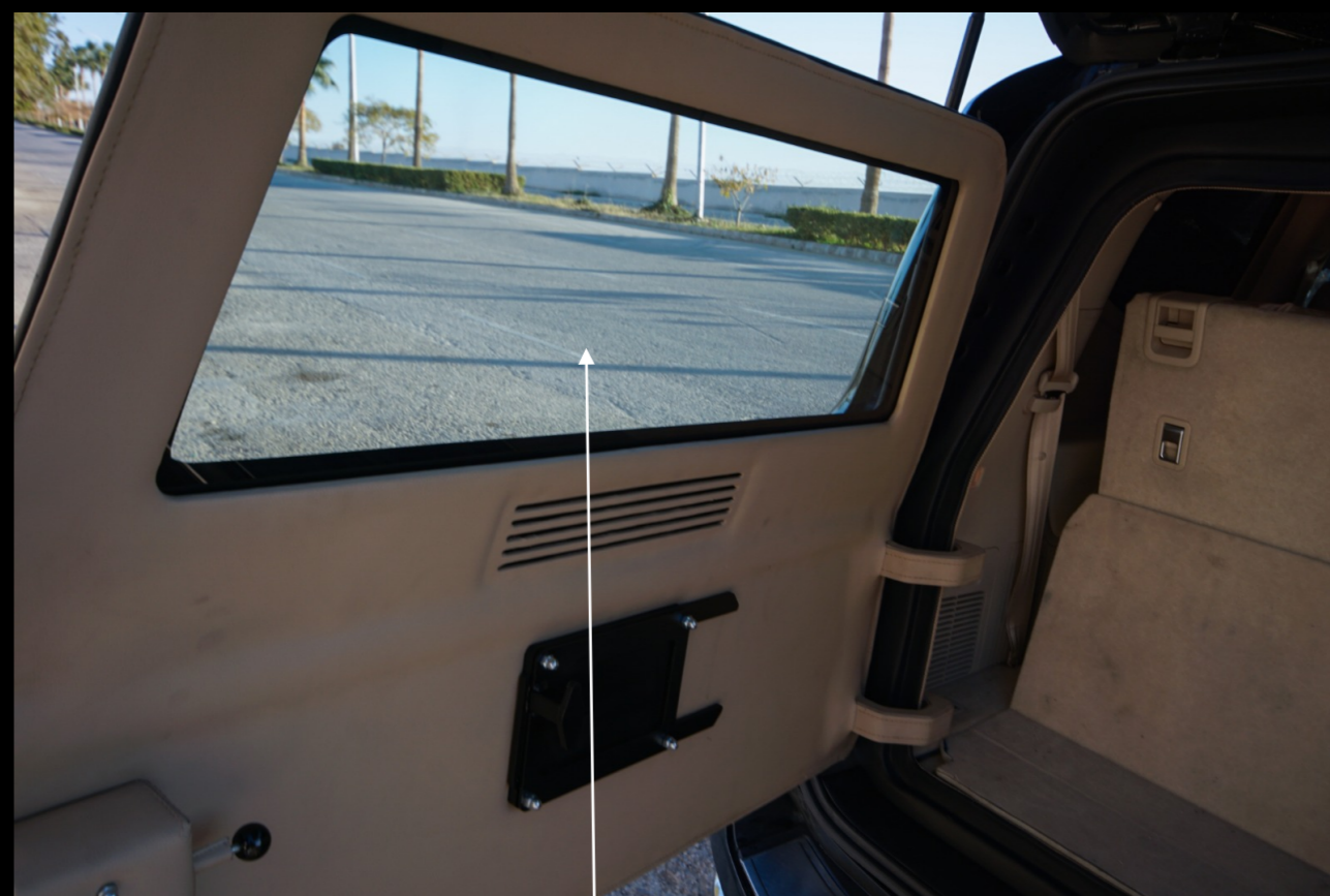
Ballistic barrier with a door and loophole with built-in laminated ballistic glass with an internal polycarbonate layer for protection against fragments inside and for an emergency exit in case of an armed attack or a traffic accident
