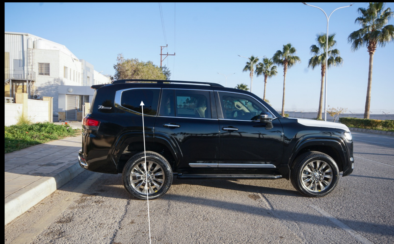
Original heated tailgate glass to bulkhead with ballistic glass and original luggage compartment side windows
