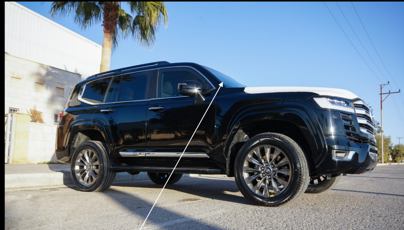
Ballistic glazing around the entire perimeter except for the glass of the rear door and side windows of the luggage compartment is made of laminated ballistic glass, including the glass of the rear partition has an internal polycarbonate layer to protect passengers from splinters inside the cabin
