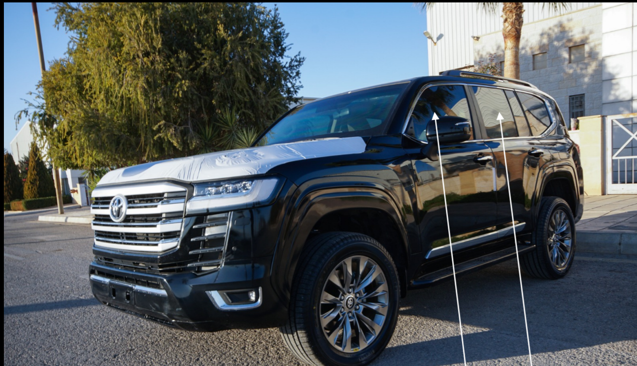
Ballistic glazing around the entire perimeter except for the glass of the rear door and side windows of the luggage compartment is made of laminated ballistic glass, including the glass of the rear partition has an internal polycarbonate layer to protect passengers from splinters inside the cabin
