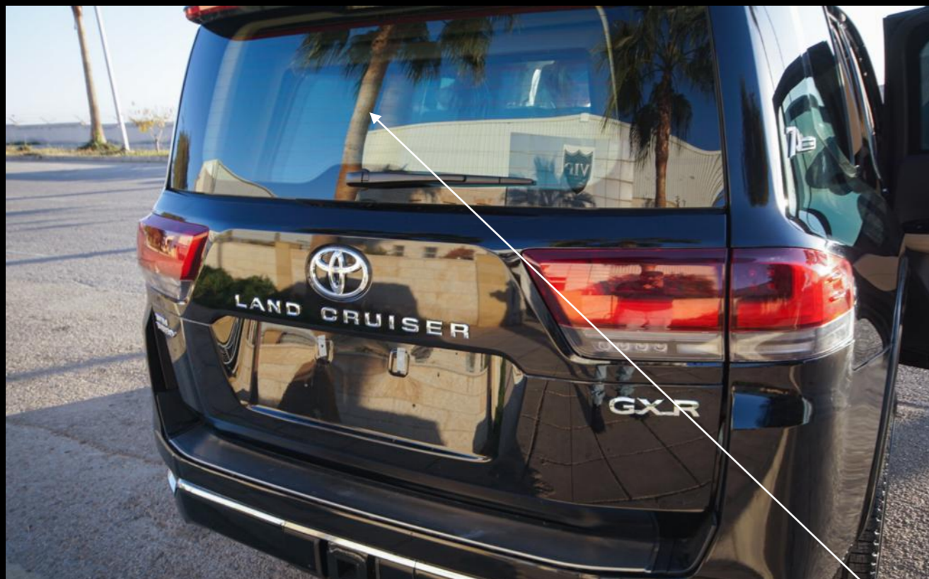
Original heated tailgate glass to bulkhead with ballistic glass and original luggage compartment side windows
