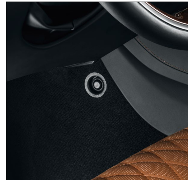
A trigger switch for the panic alarm system is located near the steering wheel.
