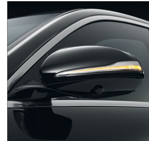
A microphone built into the flashing exterior mirror allows communication with the outside world.
