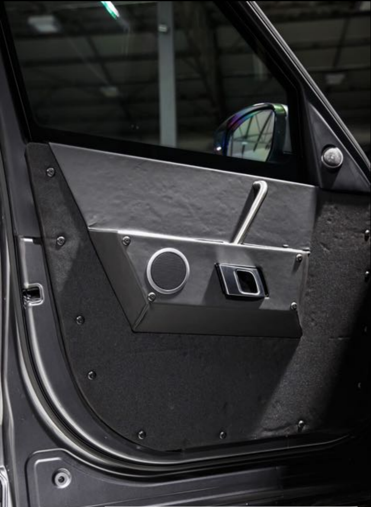
Modified interior door trim panels taking into account design features
