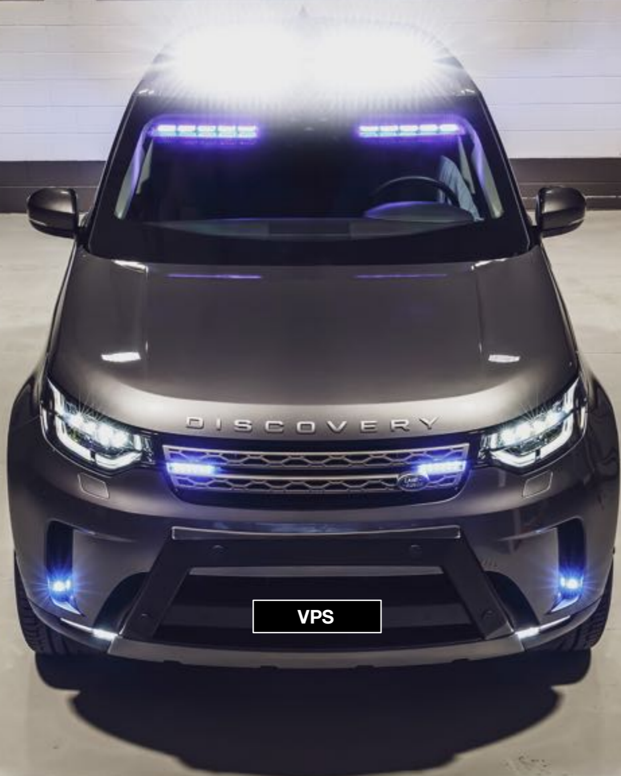
Front blue strobe lights integrated into different places
