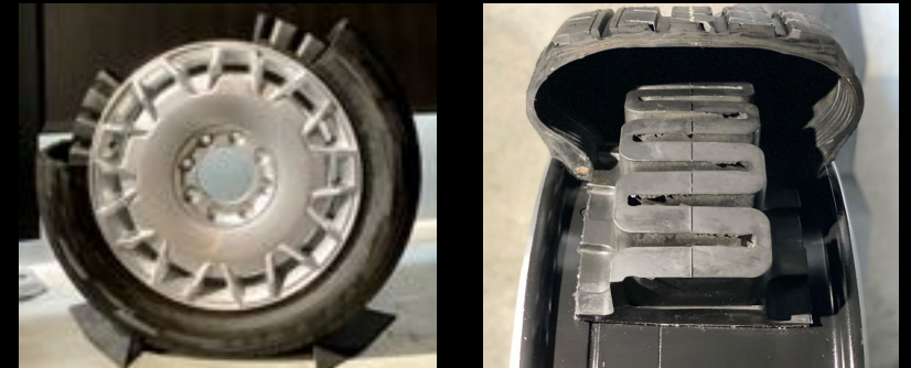
KAMA-133 tyre system with Run-flat
