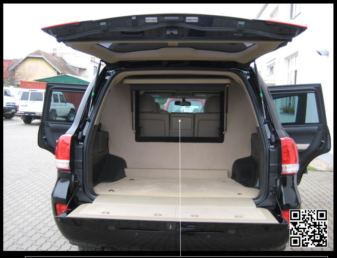
Ballistic barrier with a door with integrated laminated ballistic glass with an internal polycarbonate layer for protection against fragments for an emergency exit in the event of an armed attack or a traffic accident
