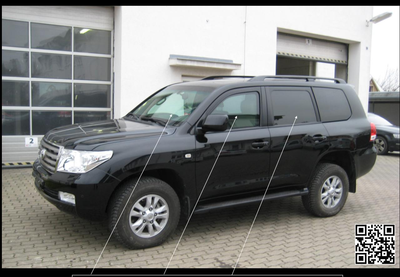
All-round ballistic glazing - except tailgate glass with ballistic glass in rear bulkhead with internal polycarbonate layer for splinter protection
