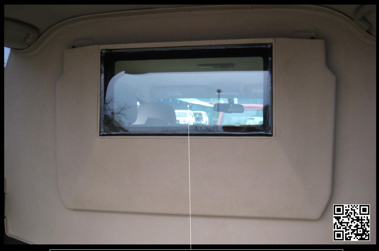
Ballistic barrier with a door with integrated laminated ballistic glass with an internal polycarbonate layer for protection against fragments for an emergency exit in the event of an armed attack or a traffic accident
