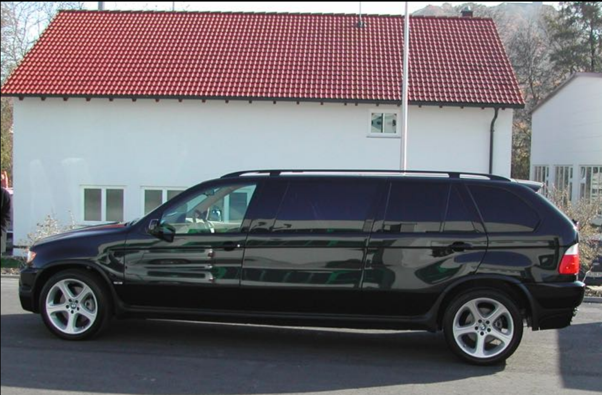
Development and production of limousine based on BMW X5+1000mm in the middle (after B-pillars) – complete car 2004
