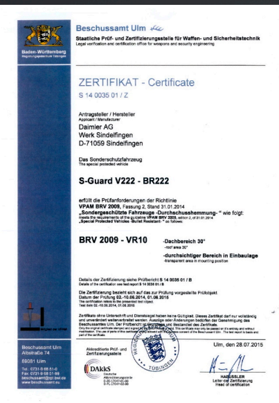
Protection against firearms - Certificate VR10 in accordance to VPAM BRV2009 directive (Bullet Resistant Vehicle)
