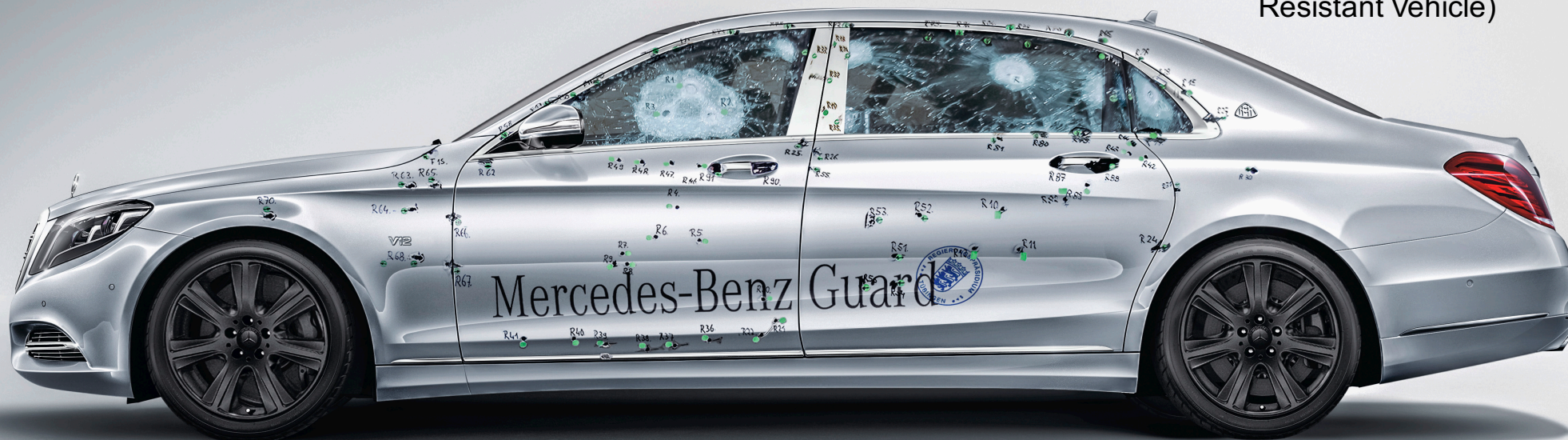
Protection against firearms - Certificate VR10 in accordance to VPAM BRV2009 directive (Bullet Resistant Vehicle)
