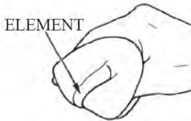
3. Reinstall the air cleaner element and the cover.
