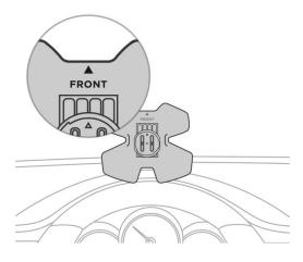
Try finding the best place for the device on your dash prior to removing the protective sheet. Using the hex key you can loosen the sliding disc screws to move it and adjust the tilt angle of the device.
