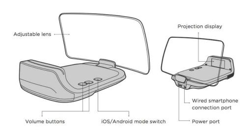
HUDWAY Cast features foldable plastic lens which receives projection from a built-in projection display and creates a virtual image focused in about 2 meters in front of the device.
