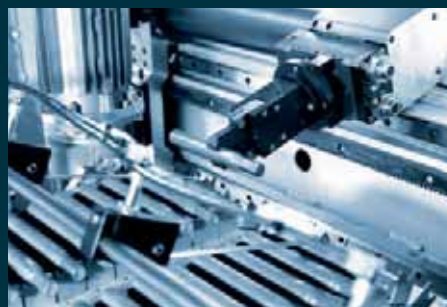
Chain feeding system with V-supports for preformed shaft parts of various shapes.
