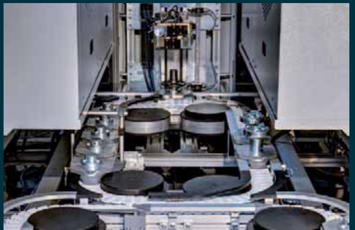
An integrated bypass line allows both simultaneous production of different workpieces, and different voltages for OP 10 and OP 20.
