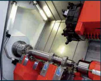
**Steady rests** / **clamping:** High-precision complete machining is possible with 3 steady rests on two process-driven slides. Optimal productivity with maximum flexibility is provided due to a shaft-chuck with retractable jaws carrier and face driver, as well as tool calibration.
