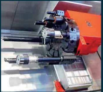
**Processing options:** The MT110 with VDI50 and block - tools can carry out optimised machining processes of short cylinder tubes with a surface quality of RA 0.2 by means of roller burnishing tools. An 80 bar band filter / coolant preparation increases the coolant volume as well as the quality and service life of the cooling lubricant.
