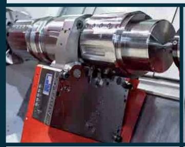
**Automatic steady rests:** Self-centering steady rest with hydraulic actuation. Built on the tailstock track and movable over Z-slides optionally movable with servo drive (NC-axis). Sealing air, central lubrication, flushing and integrated flushing channels on the arms (optional) are available for one or more steady rest units or slide systems.
