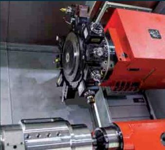
MT 110 BMT turret. For cost-effective production of complex turning/milling work pieces, in which milling is predominant, the optional BMT 65P turret with water-cooled direct drive is available. With a maximum of 9600 rpm, 56 Nm and 17.6 kW, this turret offers optimum conditions, stability for complete machining and maximum productivity.
