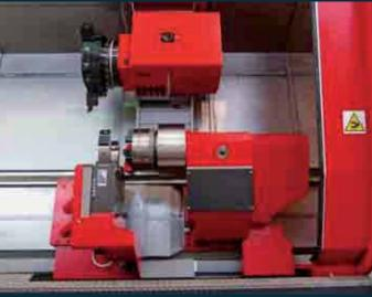
**Emco special solutions:** The Emco expertise in engineering and solutions are unique, economical and future-oriented. The standard tailstockis complemented with a 3 quick jaw change power chucks to the customer partsaccurate and stable to run / support. With the sleeve the jaw movement isprepared and everything 100% with automatic safety work state.
