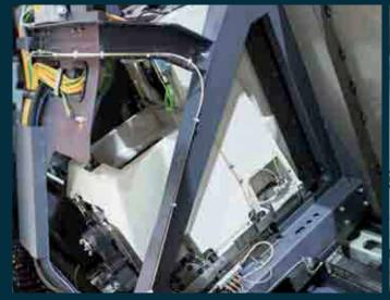
**High-precision Y-axis:** The Maxxturn machine concept has been specially developed for placement of the Y-axis at an angle of 90°. Due to large dimensioned, widely spaced and pre-loaded guide ways, the Y-axis offers optimal machining results with maximum stability and short overhangs.
