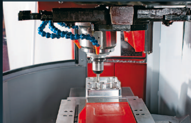
Dual-gripper arm and 'random' tool selection; mechanical spindle with high performance drive - 10000 rpm with 6,8 kW.
