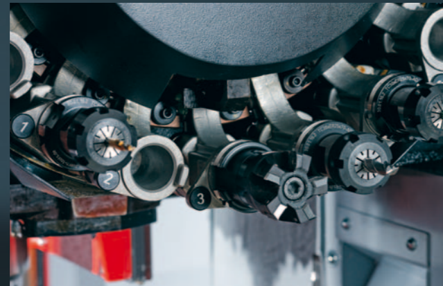
Drum-type magazine with 20 tool positions
