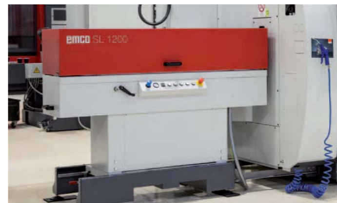
EMCO short bar loader. In view of the ever-increasing pressure on floorspace for machines, EMCO has developed the most compact short loader on the market: the EMCO SL1200.
