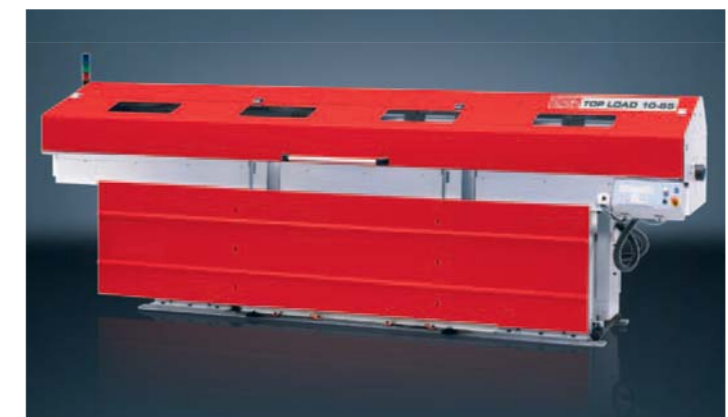
EMCO Top Load 10-65. 3-metres of bar material may be loaded into the machine in a fully automated way. Multi-Level material supports enable unmanned operation for an even longer period of time.
