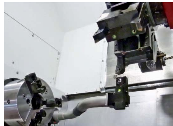
Tool measuring. The tool measuring arm equipped with a touch-probe enables fast and precise measuring of tools in the workspace. It is mounted manually in the bracket below the main spindle and returned to a storage tray after use.
