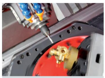
**Swivel range.** With  $\pm$ 100° swivel range the B-axis provides a larger work area compared with the products from other manufacturers. The C-axis can be rotated by 360° without limitation.
