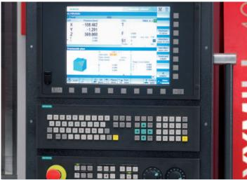
**Sinumerik 840D sl inkl. Shopmill.** Sinumerik 840D sl incl. Shopmill: The Sinumerik 840D sl incl. Shopmill is a universal and flexible CNC system and offers free contour programming, Moving cycles for complex contours, fast reference point setting with touch probe systems, tilting the working plane, Cylindrical surface machining, 3-D tool compensation, fast execution through short block processing times.
