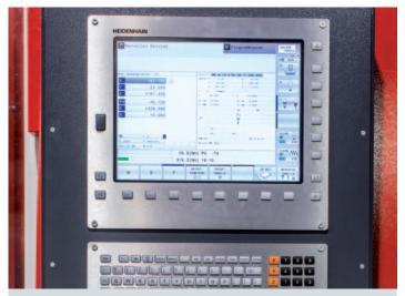
**Heidenhain TNC 620.** The latest control offers beside the milling operations also combined milling and turning operations. It is particularly suitable for Mill-Turn, HSC- and 5 axis operations at machines up to 18 axes (available only in the torque version).
