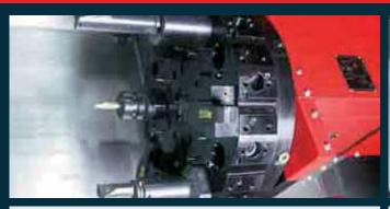
**Tool turret:** 12 + 12 station hybrid tool turret - VDI40 + block-tool, axial turret with single-motor technology. A servo motor powers the driven tools and the swivel movement. No tool rise, continuous switching with directional logic. Each station can take up driven tool holders with DIN 5480 coupling. 12 additional block-tool interfaces allow the use of large and heavy boring bars up to a diameter of 50 mm.
