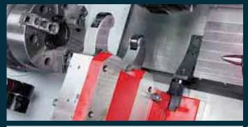
**Steady-rest.** The hydraulic operated self-centering steady-rest has a clamping range of o 30 – 245 mm. It is mounted on a slide, which can be positioned via the Z-axis-slide or optionally via an additional servo drive using a ball screw. At the determined position the slide is hydraulically clamped. The steady-rest includes chip protection and central oil lubrication.
