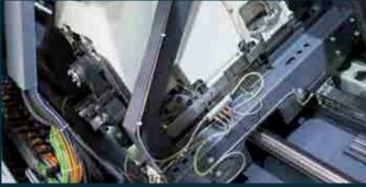
**Y-axis.** The Y-axis forms a highlight in the MAXXTURN series. She is integrated in the machine structure so that maximum stability based on short overhangs and wide distanced roller guids is guaranteed. Thus, complex machining tasks can be done and workpieces can be completely finished in a single setup. A variety of machining cycles in the controller allows easy programming and the use of the additional linear axis.
