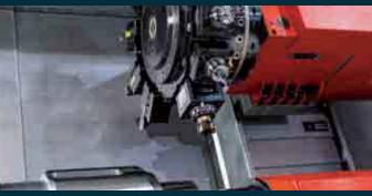
**BMT turret.** For cost-effective production of complex turning/milling work pieces, in which milling is predominant, the optional BMT 55P turret with water-cooled direct drive is available. With a maximum of 12000 rpm, 30 Nm and 10 kW, this turret offers optimum conditions, stability for complete machining and maximum productivity.
