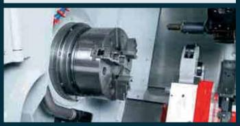
**Main spindle.** Two versions are available. One using a conventional beld-drive for high torque (up to 1040 Nm) and heavy machining and another one using the approved water-cooled motor spindle for higher spindle speeds. This one also offers optimal conditions for complex milling operations.
