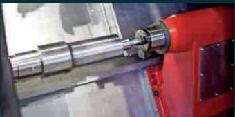
**Tailstock.** The tailstock is mounted on linear roller-type slides and can be positioned via the z-axis-slide. Optionally an additional servo drive using a ball screw can be offered. At the determined position the slide is hydraulically clamped. So that a quill with integrated bearings and MT4 cone can support the workpiece. Therefore the quill can move up to 120 mm.
