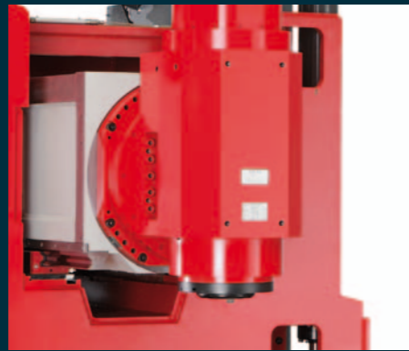
Milling spindle: The machine is equipped with a liquid cooled motor spindle with compelling performance specs. At spindle speeds of 15000 rpm, a power rating of 46 kW, and a torque of 170 Nm, the machine is also suited for heavy-duty machining. A motor spindle 18000 rpm is available with HSK A63.
