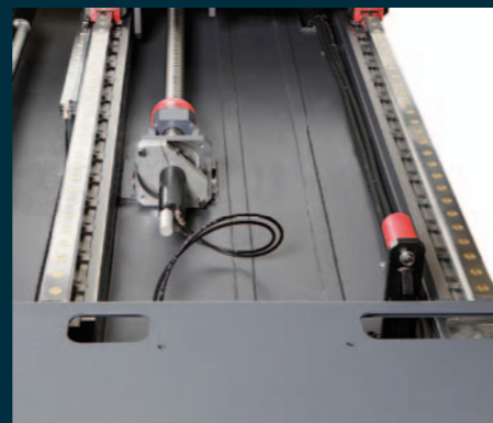
Axis drives: Linear axes are equipped with linear guides. Long way-guides are used to attain the necessary rigidity. The drive is equipped with a ball screw drive with direct drive bellows coupling. The direct drive provides for highly dynamic axis travel, while also employing a low maintenance and smooth drive system. The X-axis linear scale is standard due to the long travel.
