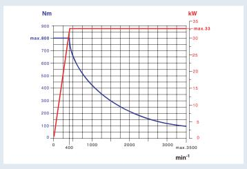
Main spindle A2-8 - counter spindle A2-8
