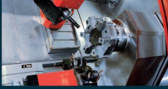
Counter spindle view with 6-position jaw chuck  $\emptyset$  500 mm. The upper turret is replaced by a 21 kW liquid-cooled milling spindle in the B axis version. The B axis travel range is 205°. This is infinitely variable with 0.001° resolution. In addition, the B axis can be clamped in any position with 5° indexing.
