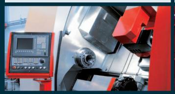
The work area provides the highest level of ergonomics with excellent accessibility to the individual components. Generous amounts of free space ensure optimal chip flow, even when machining complex materials. All guides are covered in stainless steel sheets to prevent damage.
