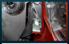
Parts catcher with conveyor: Finished parts are ejected with a coolant fed part ejector into the parts catcher and transferred with a conveyor to a storage area.
