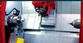
The modular machine concept also enables the use of a tailstock in combination with an NC-controlled steady rest instead of the lower tool turret, depending on the customer's requirements. The steady rest can be hydraulically lowered 250 mm if required.
