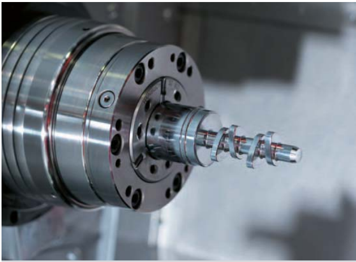
Main spindle. The 15 kW motor spindle with its integrated water cooling system provides high dynamics but low thermal displacement. A high-resolution shaft encoder provides the optimum conditions for accurate contour milling and drilling.
