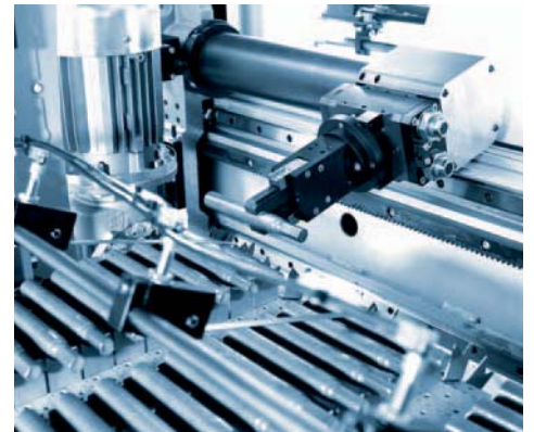
Timed conveyor system with V-supports for preformed shaft parts of various shapes.
