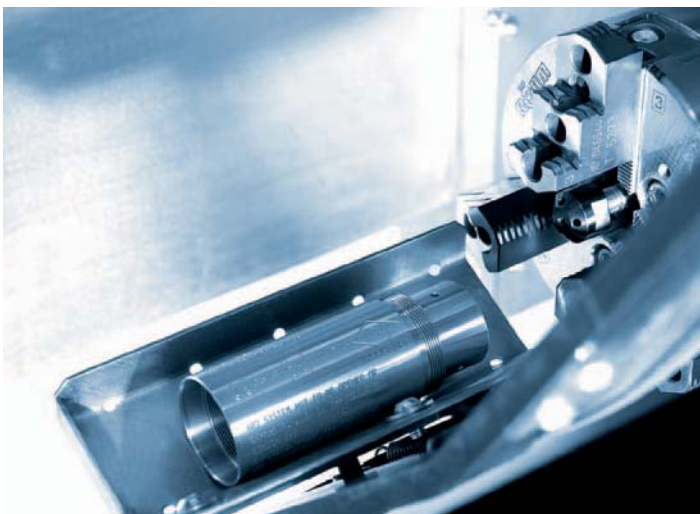
Parts catcher. The HYPERTURN 45's pneumatic parts catcher is controlled using M-functions. When needed, it traverses to the front of the work area and travels to the spindle center. The finished part is removed from the clamping device and transferred to the catcher tray. The parts catcher then moves back to its initial position and the part is tipped into a catching box or onto a conveyor belt.
