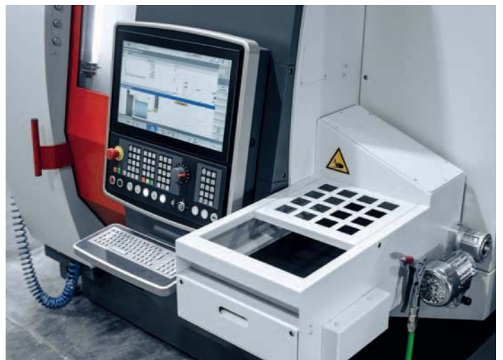
Finished parts conveyor. The parts catcher deposits the finished parts on an accumulating conveyor with a usable storage area of 340 x 750 mm. Since the belt is clocked, the parts – which are often very complex – are kept from falling on top of each other.
