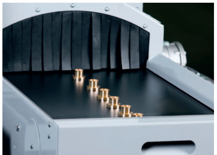
Finished part conveyor. The finished-part pick-up device puts the parts on an accumulating conveyor. A discontinuous belt ensures that the often very complex parts do not fall onto each other.
