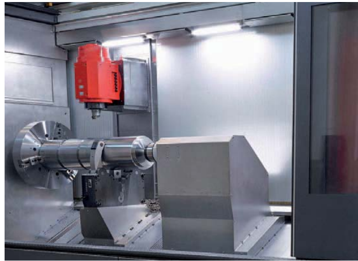
Main spindle. For turning and milling operations, equipped with 84 kW and 6400 Nm torque. Sealing air, working area coolant and programmable clamping pressure are standard features on the Hyperturn 200. One or more programmable NC steady rest can assist the processing.
