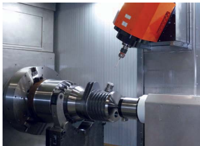
Tool measurement. The entire tool measurement is integrated in the process and guarantees high precision as well as measurements during the machining process.
