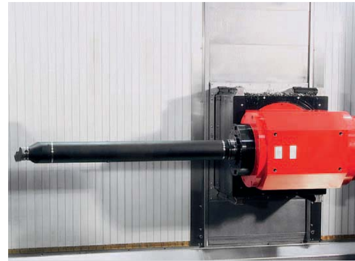
Turning operations. External or internal turning operations are possible with the stable spindle in 3° step. Optionally, the vibration-damped boring bar can be equipped up to a length of 1000 mm and with a 3-positions (stations) pick-up magazine.
