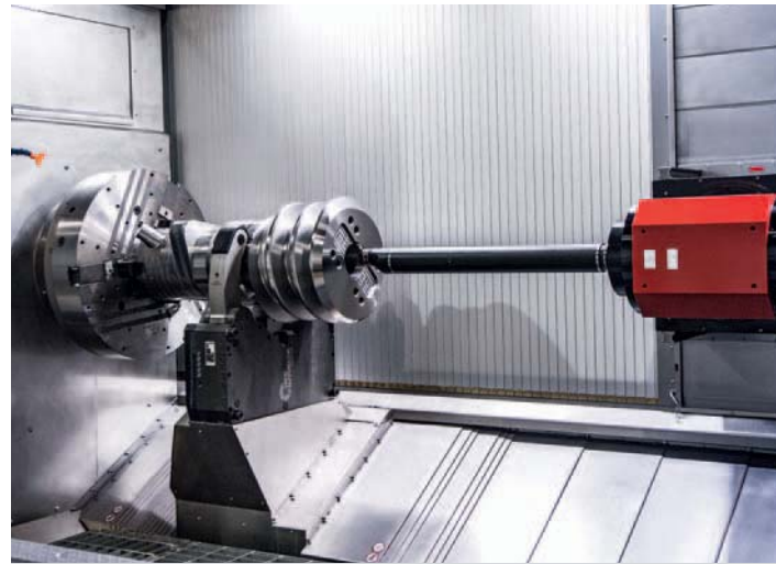
Boring bar: Boring bar with vibration absorption featuring a diameter of 100 x 100 mm for internal turning operations. There are three specifically dimensioned tools available.
