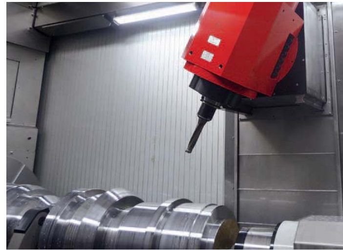
Milling spindle. For stable, precise and flexible drilling and milling operations. Up to 80 kW and 630 Nm of torque and 10000 rpm. Sealing air, internal HP coolant with 40 bar and externally with 14 bar and a 1400 liter paper band filter system as standard (80 bar option). The B-axis can be used at any angle or with an indexed B-axis in 2.5° steps.
