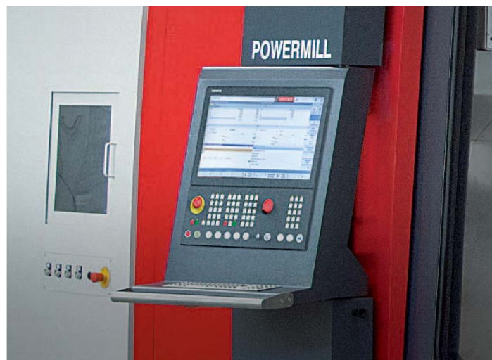
auriga's hardware basis is a 22" industrial touch control panel combined with an industrial PC (IPC).
