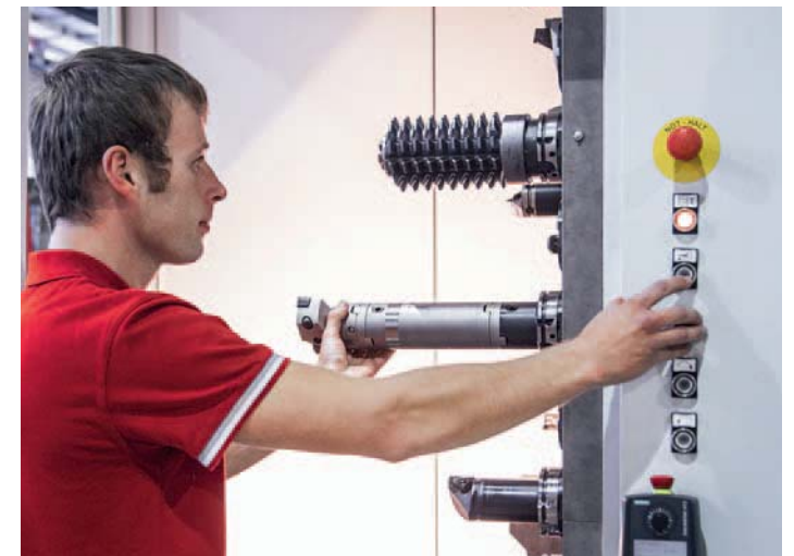
Ergonomic loading of the tool magazine with tools weighing up to 25 kg and measuring more than 600 mm
