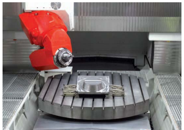
15° undercut. The milling head with 15° undercut allows for added value in complete machining in one setup.
