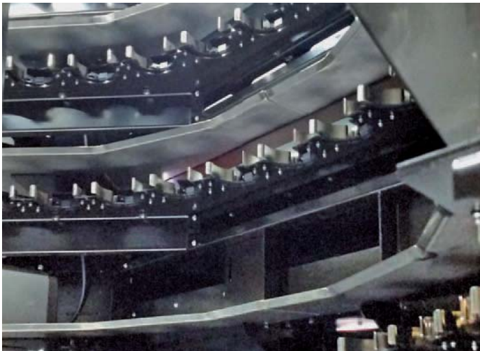
Tool loading and unloading. Operators use the foot pedal to unload and load the tools, thus having their hands free for their activities on the machine.
