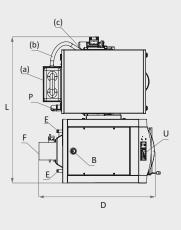
Combined boiler WBS AC-UB; (2) Fuel hopper UB; (3) Safety heat evacuator; (4) Turbulators;
