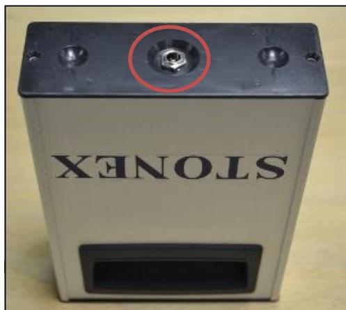
Figure 9: Battery power plug
