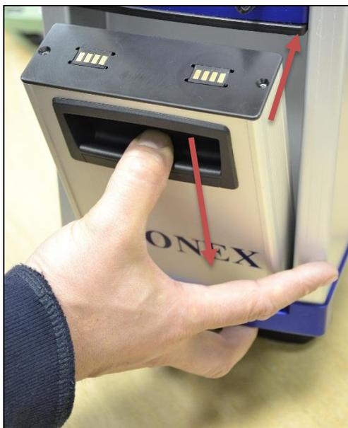
Figure 5: Plug the battery pack
