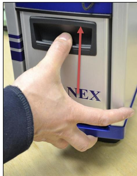
Figure 6: Plug the battery pack
